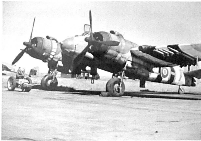
43. A Beaufighter at Davidstow Moor armed with rocket projectiles in addition to cannon. In the foreground is a 'trolley ac' used to start aircraft engines to save using the aircraft's batteries.
