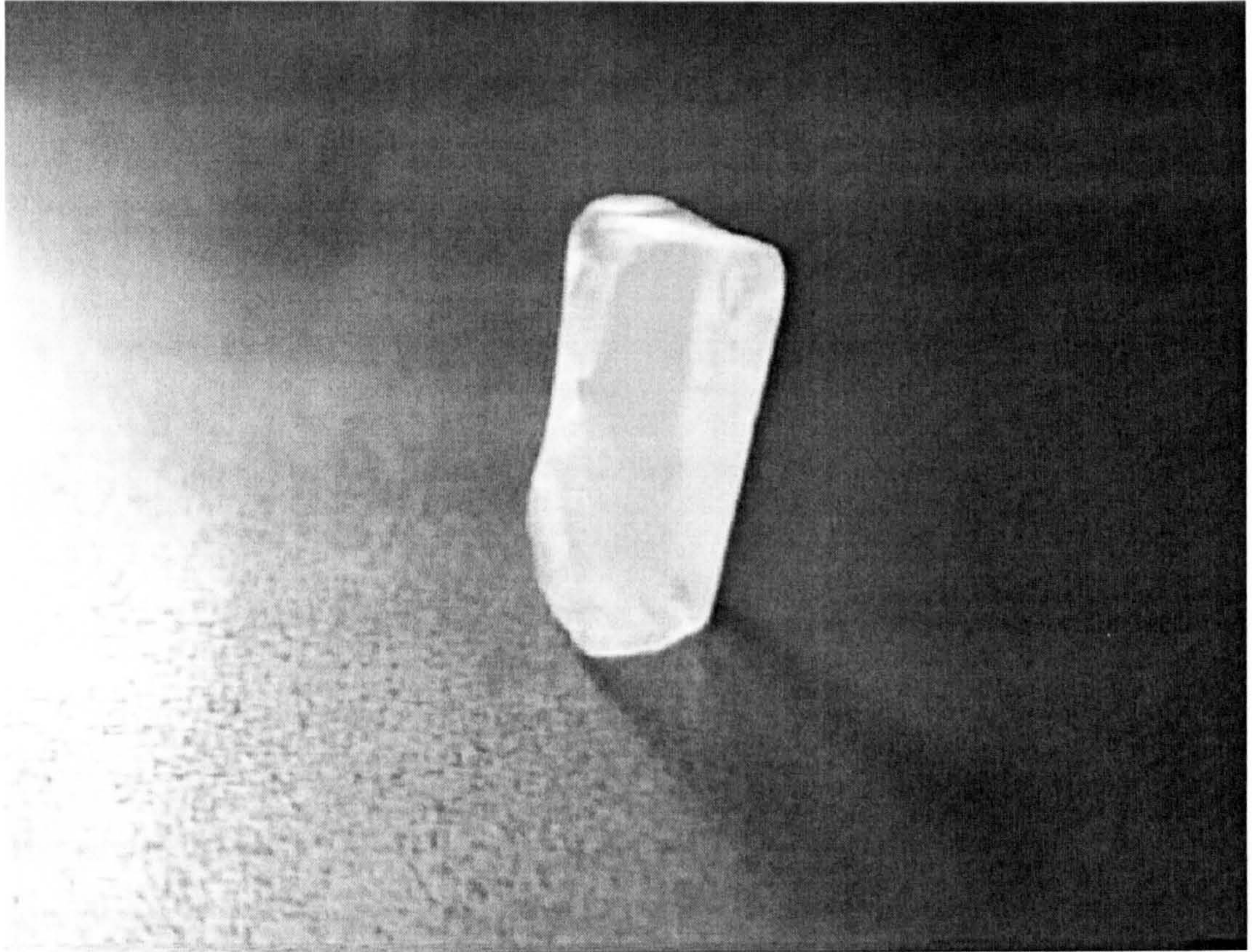
Figure 1.5 shows a typical bulk aerogel for use in industry
