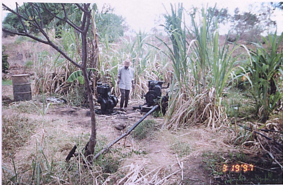
Figure 5.4a Diesel pumps used for crop irrigation along Voi River. Notice the pumps in the open among sugar cane plants.
