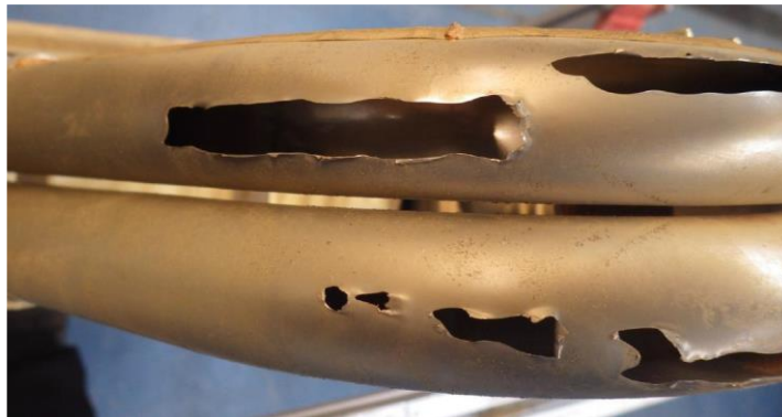
Figure 2.9 Excessive erosion in the outlet side of Coriolis tubes [11]
