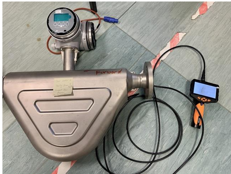
Figure 5.22 Photo of visual inspection of the meter under test (CF2)
