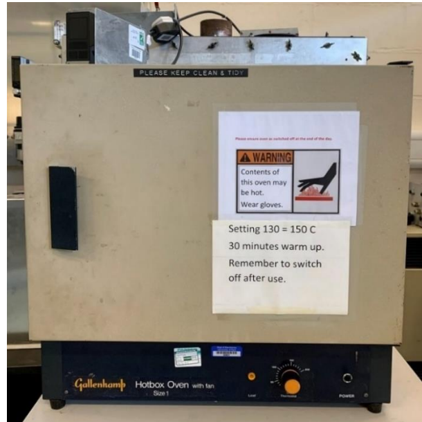
Figure 3.17 Heating oven to dry wet sand
