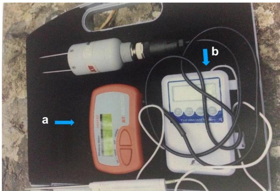
**Figure 2.9** Machine for measurement of (a) soil temperature and (b) moisture content
