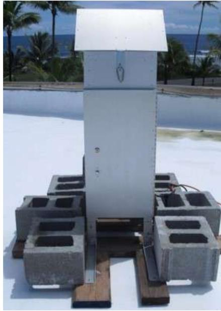
**Figure 3.1:** The Kwajalein micrometeorite collector in position on the Kwajalein atoll. The breeze blocks are to hold the collector in position.
