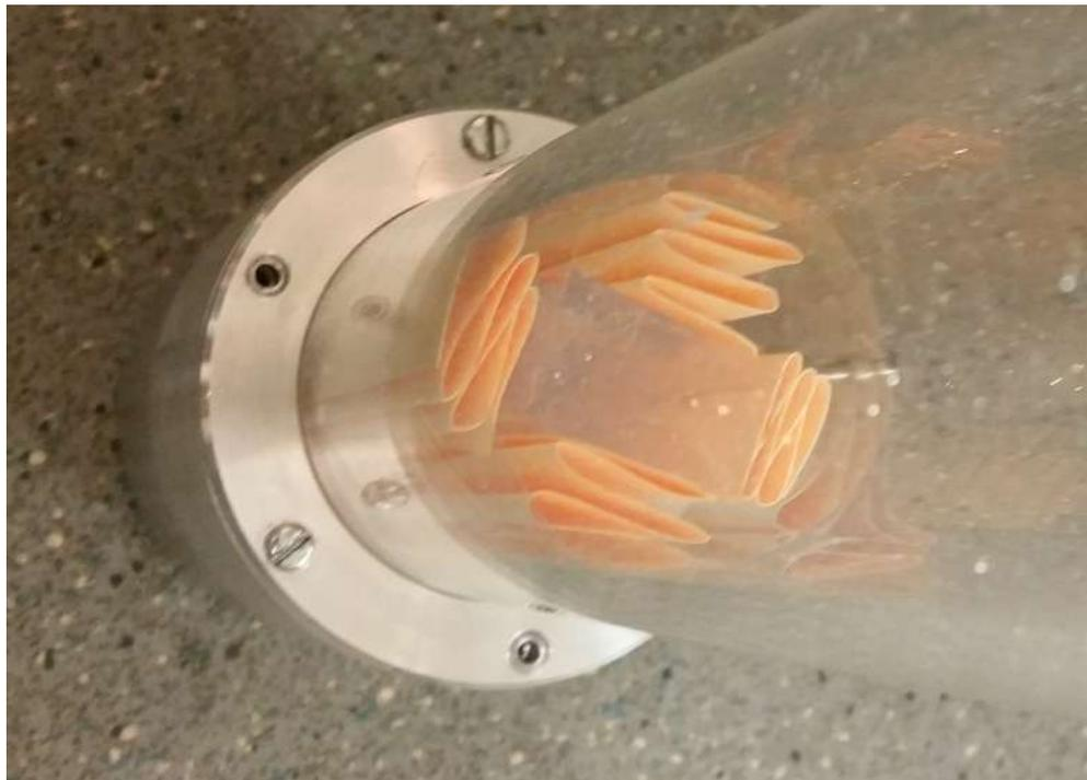
**Figure 6.1:** The loaded capture medium cartridge (Mylar walled) in the EVT.
