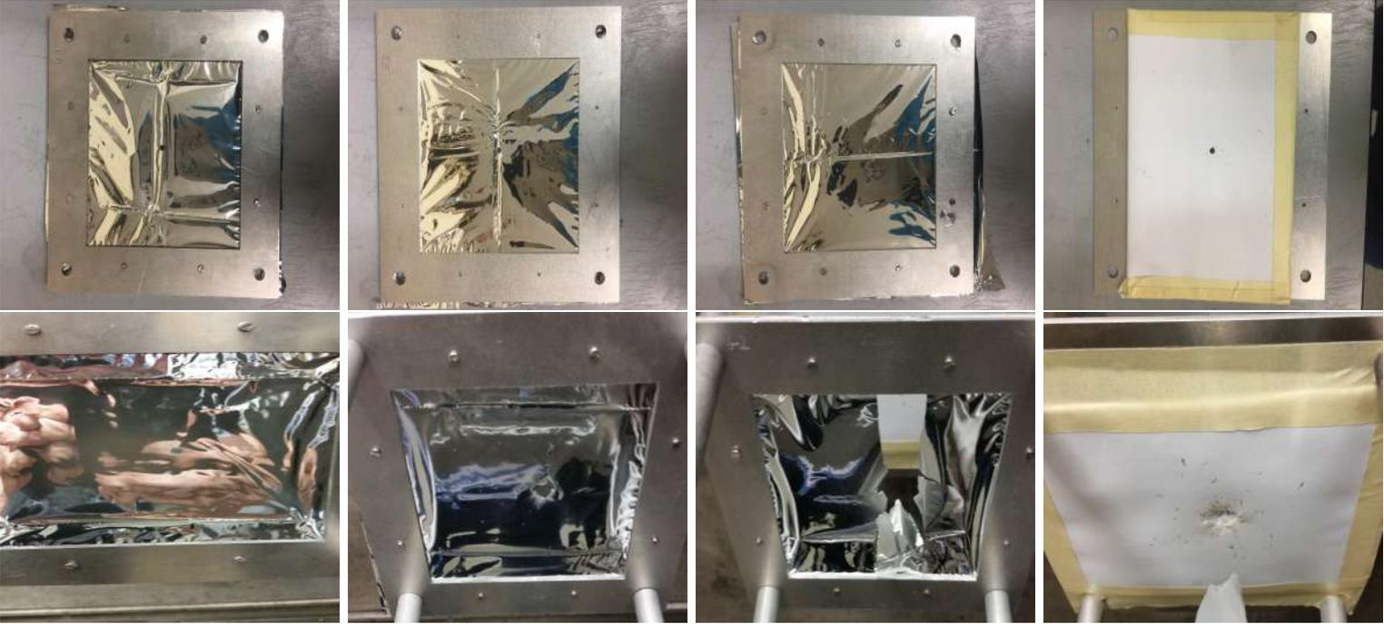
**Figure 6.16:** Photographs of the foils and paper stoppers after shooting in shots 4 (top row) and 5 (bottom row). Foils progress front to back from left to right. In shot 4 the holes in the foil do not increase in size, however in shot 5 the size rapidly increases. The small holes in both sets of foils are likely from impacts from ejecta from the previous foil.
