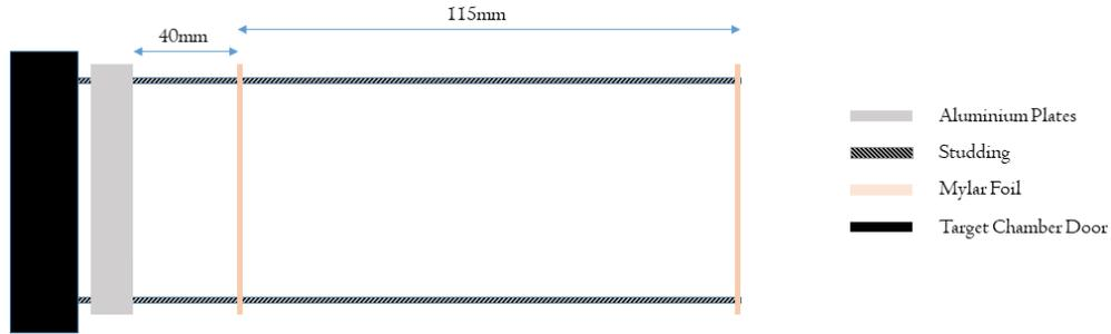
**Figure 6.14:** Schematic showing the set-up for the first foil test (shot 3) to study the effect of the Mylar foil on the peridot projectiles.
