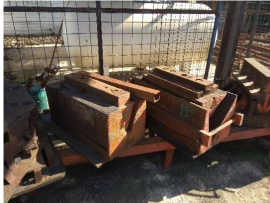
Fig. 11. Thermal processing moulds for shaping the 'wings' of the farming ploughs used by Glavanis Ironworks.
