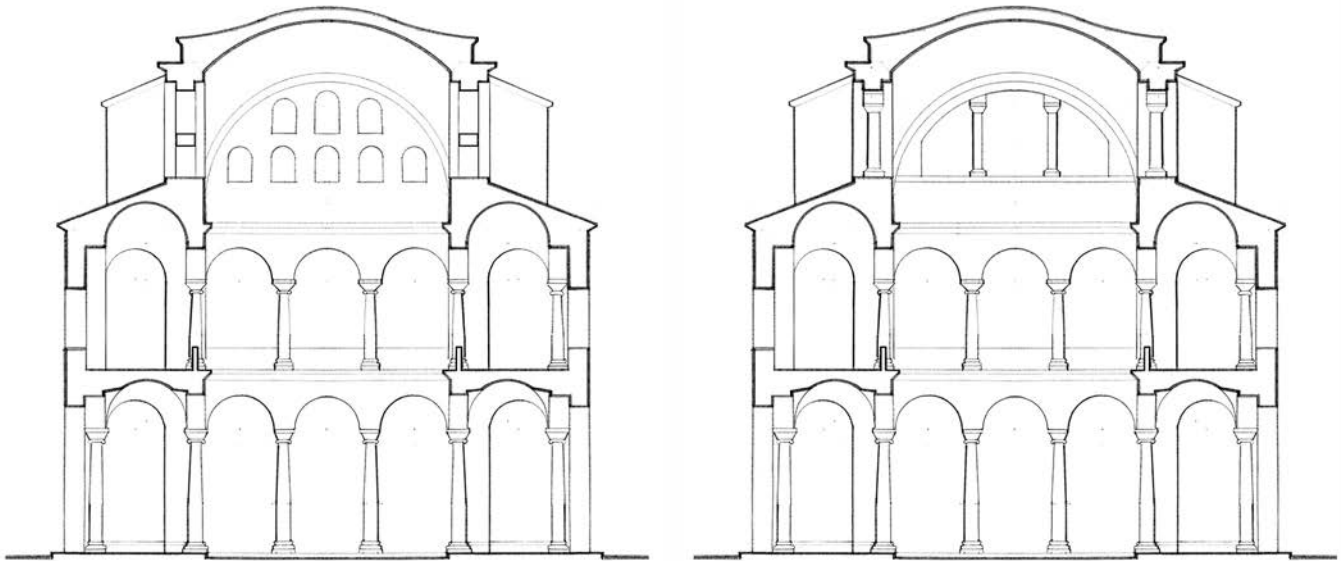
FIG. 7.12. Church of the Holy Apostles. Reconstructed cross-sections of the east cross arm, showing two alternative clerestory walls. The left version displays a window pattern similar to that of Hagia Eirene in Constantinople. The right version explores the possibility of “thermal,” mullioned windows similar to those of Hagia Sophia in Constantinople and St. John at Ephesus (drawing by author, 2016).
