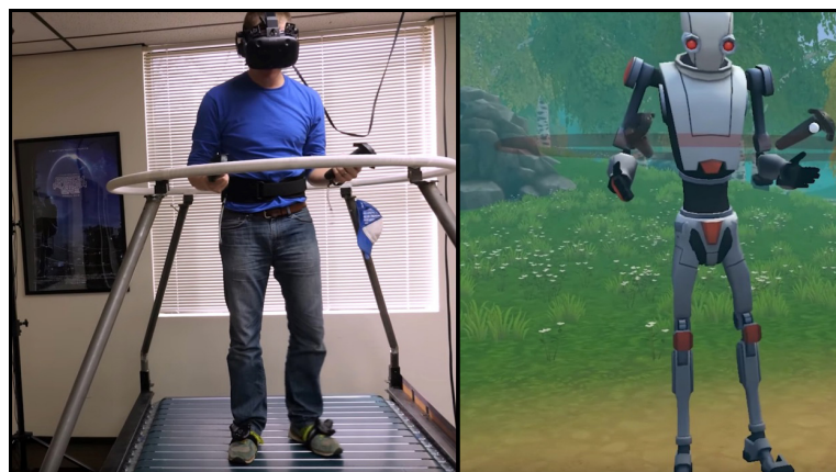
Figure 2.18: A person immersed in VR with HTC Vive and omni-directional treadmill technology (retrieved from Streeter, 2018)
