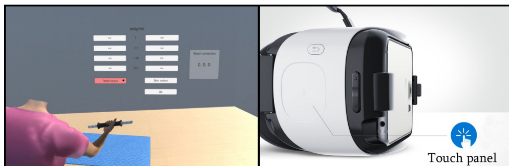
Figure 3.17: On the left a screenshot showing the process of setting up the application by the psychologist; On the right the Gear VR touch panel that the psychologist uses to simulate the mouse button click
