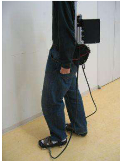
Figure 2.17: Virtual Reality Powered Shoes (retrieved from Iwata, Yano, & Tomioka, 2006)
