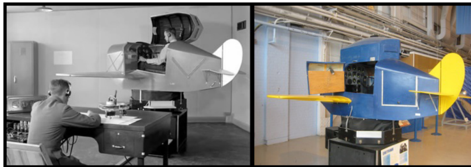
Figure 2.1: The first flight simulator “Link Trainer” (retrieved from Zuk, 2010)
