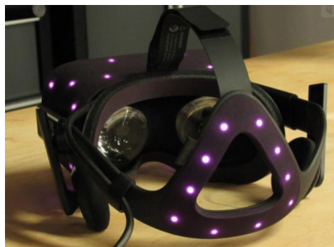
Figure 2.14: The infrared sensors of the Oculus Rift headset (retrieved from Lang, 2016)
