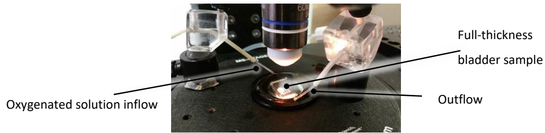
Figure 14 DIC imaging. Full-thickness bladder samples were imaged using an upright Olympus BX51WI microscope, positioned in a lens dish filled with Krebs-Henseleit buffer bath, with the mucosa facing upwards and kept in place by a harp pin. Tissue samples were continuously superfused with oxygenated Krebs-Henseleit buffer at a rate of 2.5 \text{ mL min}^{-1} . Images were obtained with an Olympus x60 water immersion objective with a Rolera XR CCD camera.
