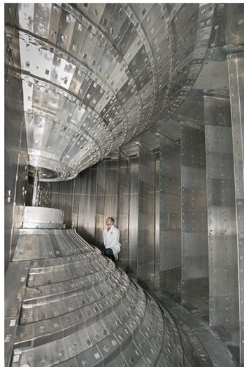
**Figure 2.14** Photograph of the inside of LET, showing the large area detectors.
