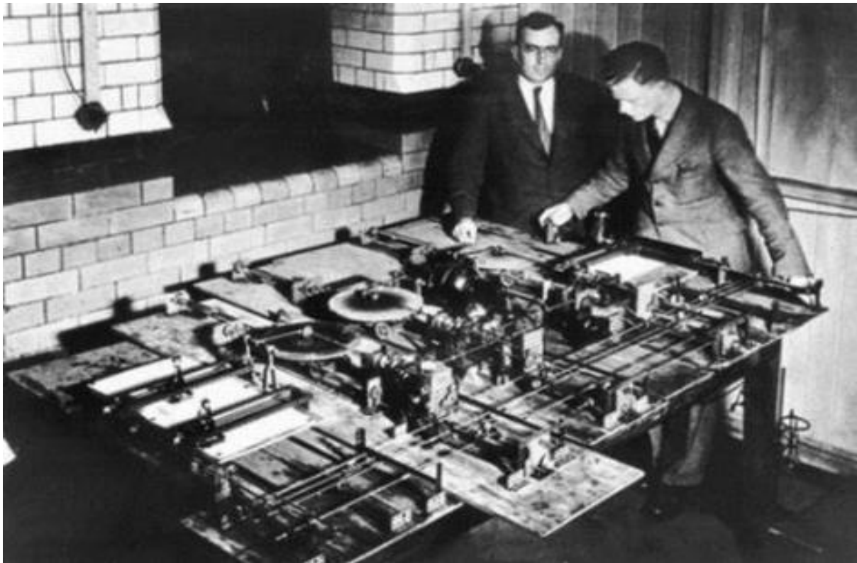
Figure 4: An image of the original Meccano differential analyser built by Douglas Hartree (L) and Arthur Porter (R) in 1934. (© Science and Industry Museum Informal Collection).
