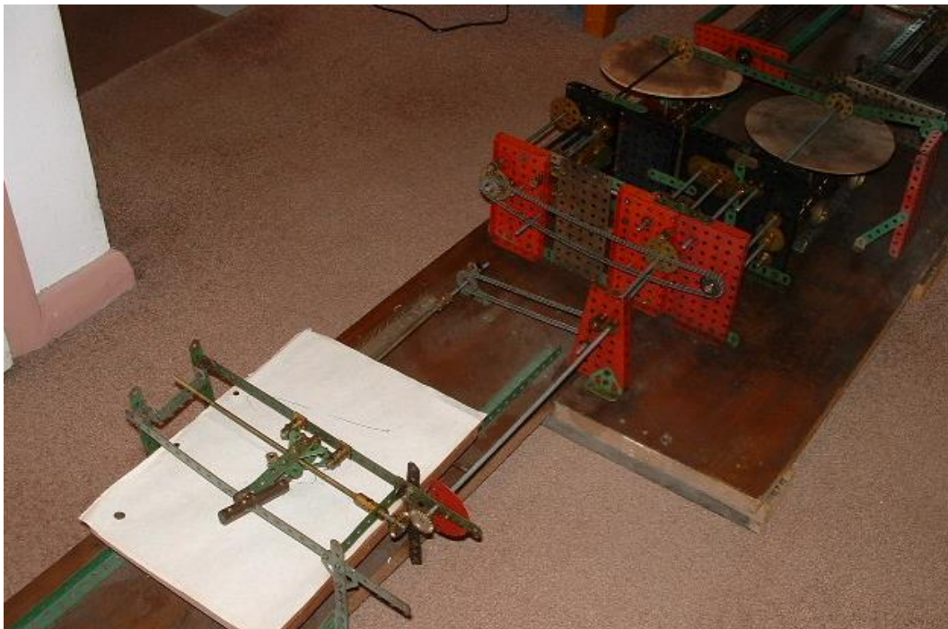
Figure 3.18: An image of the recently rediscovered two-integrator Eyres model. (Image reproduced from Eyres family personal collection).
