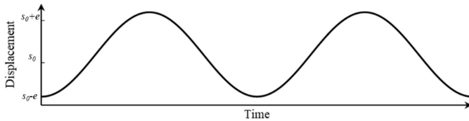
Figure 3.31 Displacement function of an eccentric shaft.
