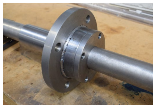
(c) Supporting/sealing flange (to be attached the existing flange of the boiler)
