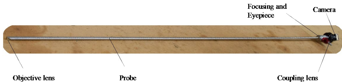
(a) Overview of the optical probe (with the camera attached).
