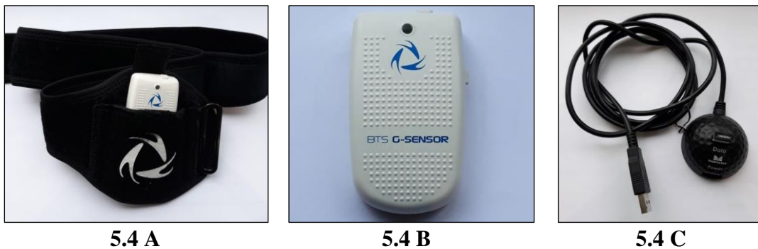
Figure 5.4 G-Walk system (G-Sensor®, BTS Bioengineering S.p.A., Italy): 5.4 A) Waist belt with a pocket for the wireless inertial sensor; 5.4 B) Wireless inertial sensor; 5.4 C) Bluetooth dongle and Bluetooth extension cable.
