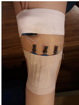
Figure 2 Stretch sensors covered by kinesiotape
