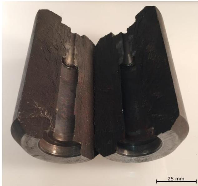
Figure 3.12: A central breech that has been split in two after being impacted by a piston at too great a velocity.
