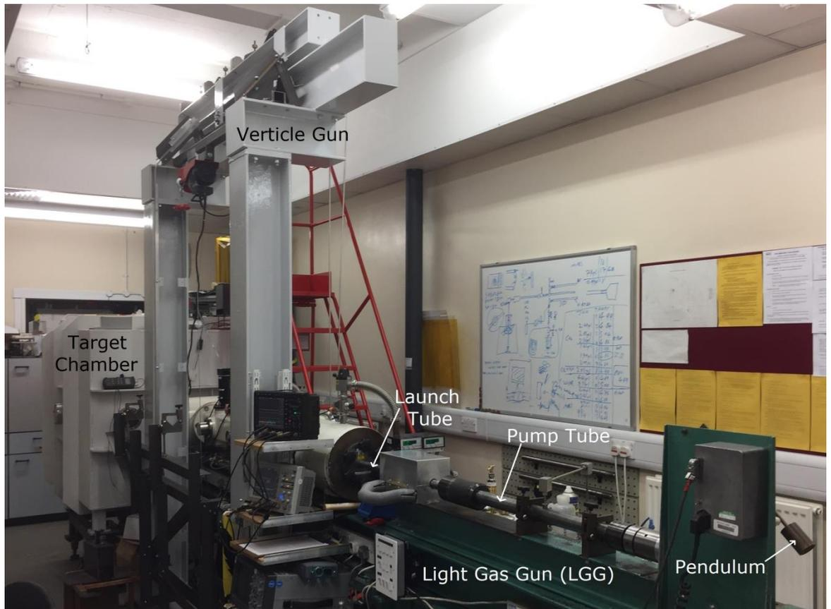
Figure 3.5: The LGG facility at the University of Kent as of November 2017
