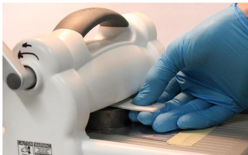
Figure 3.33: The stack of packing material being held in place while the punch being run through the Big Shot press.
