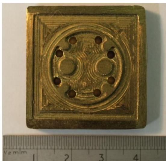
Figure 3.22: The prototype foil punch made from brass and constructed using a CNC milling machine.
