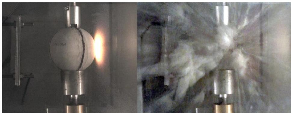
Figure 3.8: (left) A spherical target in the rotating target holder at the moment of impact and (Right) during complete disruption of the target (approximately 5 milliseconds later).
