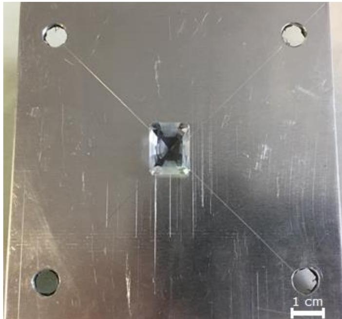
Figure 5.2 A quartz gemstone mounted to an aluminium target plate using Leit C-plast.
