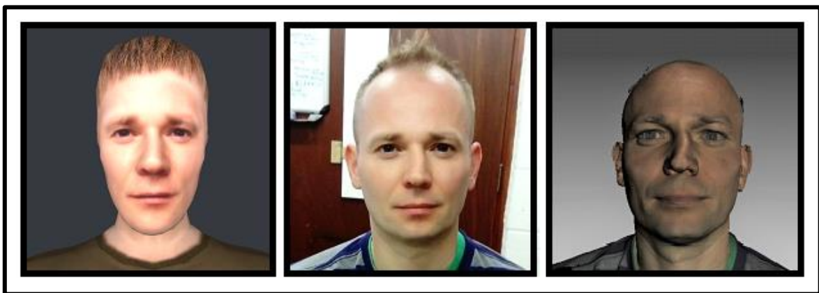
Figure 5.1. Comparison of avatar construction methods. The left image is an avatar created from the centre face photograph using the method described in Chapter 2. The photograph was taken at the time of a facial scan, the outcome of which after initial rendering is shown in the right image.
