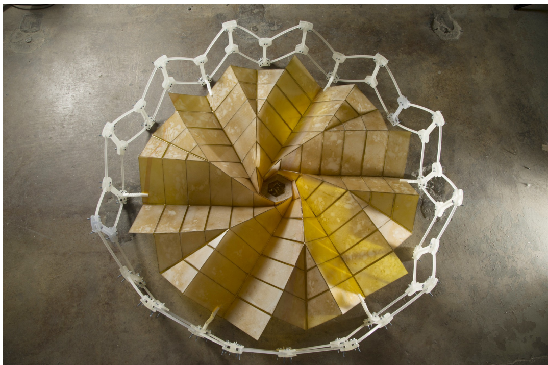
Figure 2.12: Origami Solar Panel Prototype [14]
