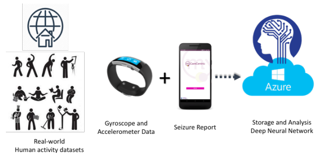
Figure 4: The system structure of the wearable data collection system
