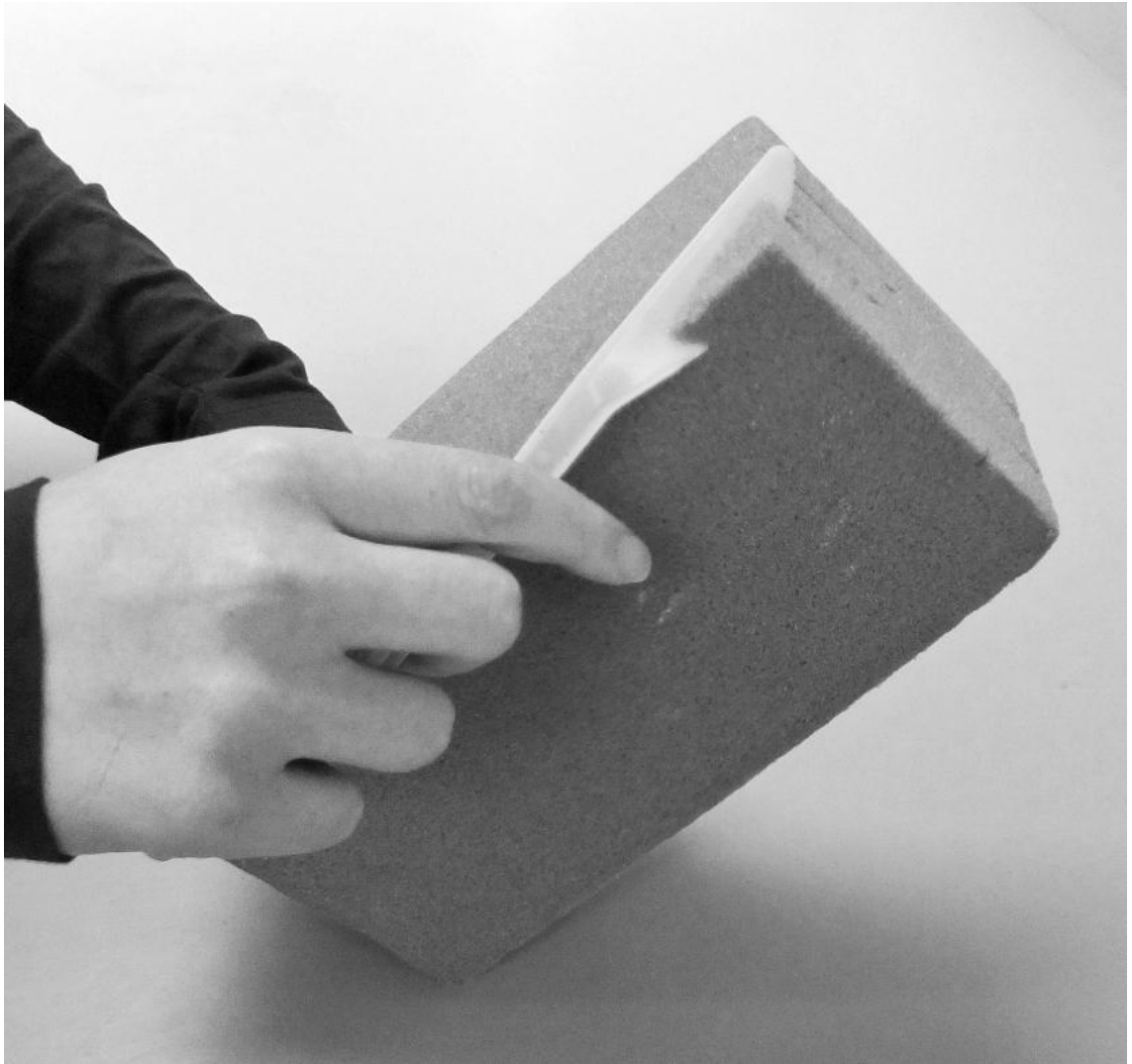
Figure 5.1: Example of cutting corners from a standardised foam block.
