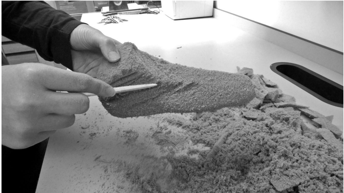
Figure 5.5: Final shaping via scraping.
