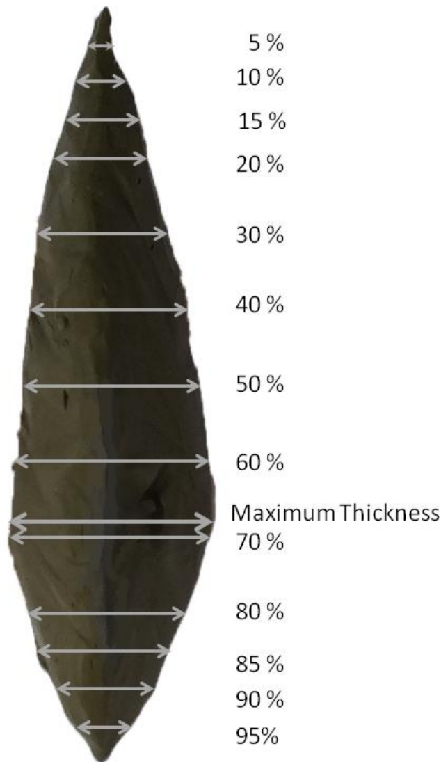
Figure 2.11: Lateral measurements taken from the maximum length line of the profile-view of a plasticine replica.
