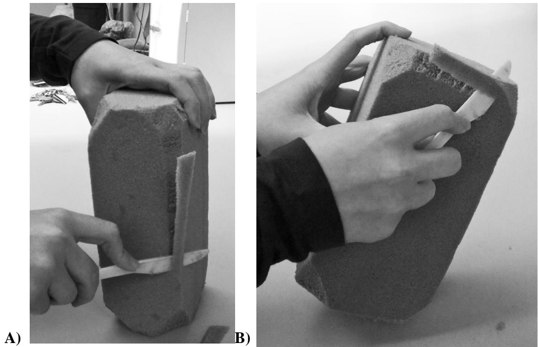
Figure 5.2: Example of cutting long margins (A) and small margins of the foam block (B).
