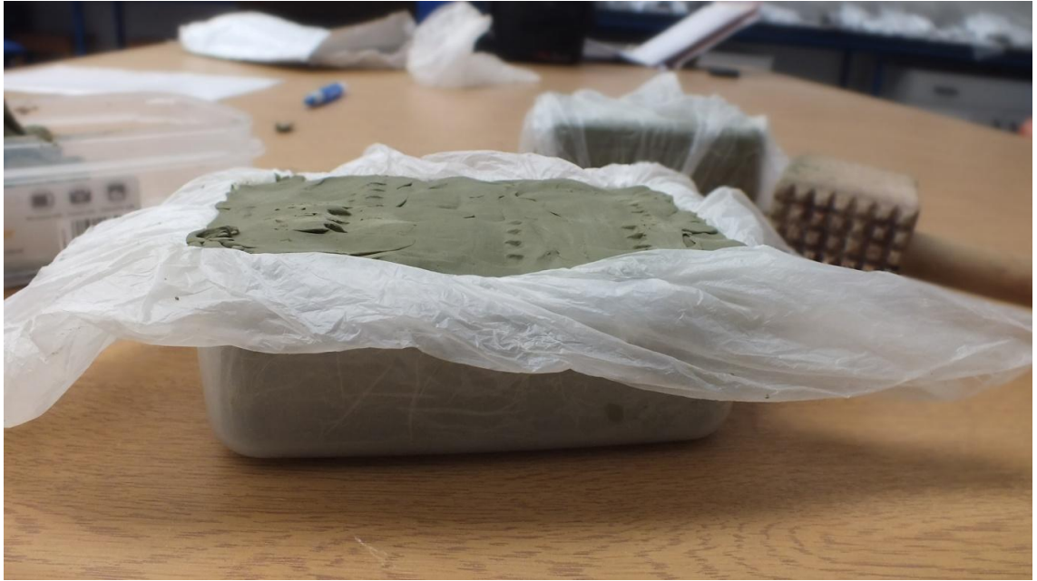
Figure 3.2: The procedure of making standardised plasticine blocks using plastic containers that measured 13.5cm in length, 8.7cm in width, and 4.5cm in depth. Thin plastic sheets were placed inside the containers prior filling the plasticine to assure the gentle removal of the plasticine blocks.
