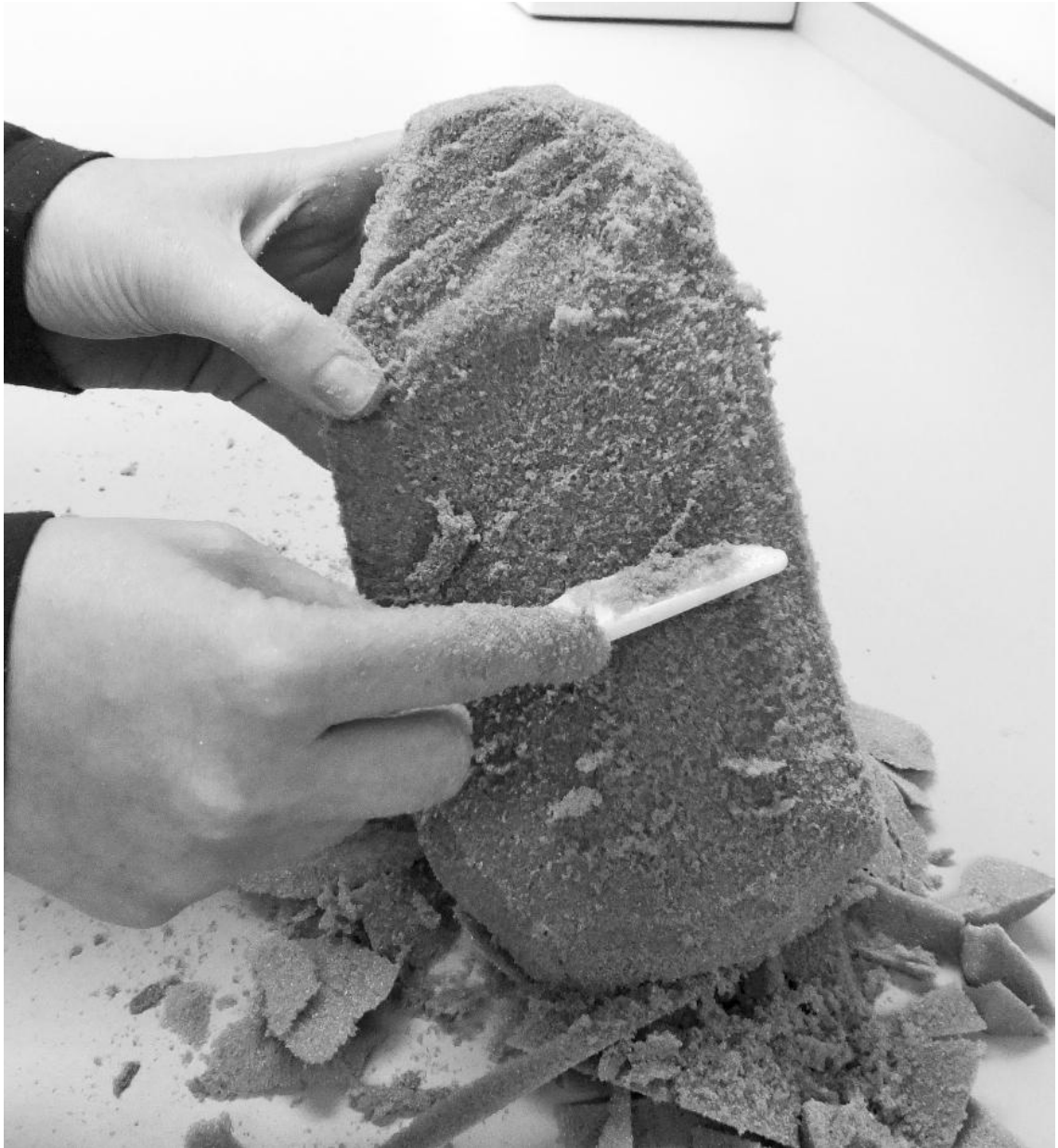
Figure 5.4: Example of scraping movements as the main technique of foam removal.
