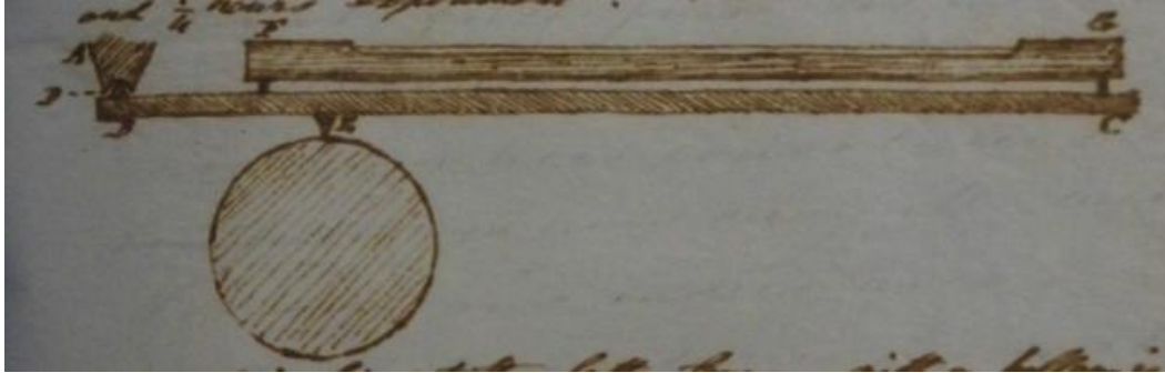
Fig. 22. Sketch made by Airy showing the instrument to check the ellipticity of the pivots (Airy to May, 4 December 1849, RGO 6/722)
