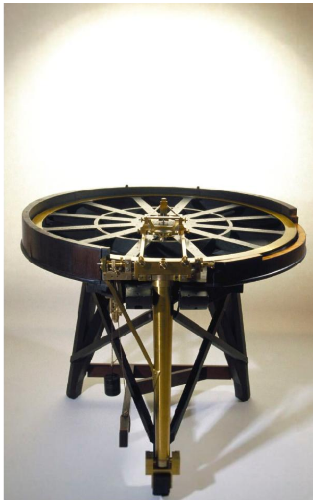
Fig. 17. John Troughton's Dividing Engine (Science Museum, Object number: 1932-22)
