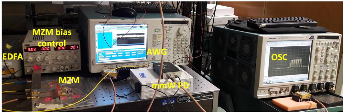
Figure 6-10 External IM-DD experiments (Top: schematic; Bottom: actual laboratory testbed) at RF with DMT and SSB modulated multiplexes using a single IFFT and generic numerologies (device models and parameters shown in Table 6-2).
