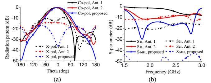
Fig. 3. Simulated results of the antennas in the evolution process. (a) Radiation patterns at 2.2 GHz in V-plane. (b) S-parameters.
