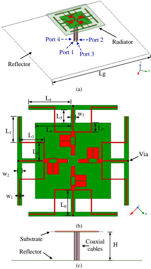
Fig. 1. Configuration of the proposed dual-polarized antenna. (a) Isometric view. (b) Top view of the antenna radiator. (c) Side view. (Detailed parameters of the proposed dual-polarized antenna:  $L_g=140$  mm,  $L_0=11.5$  mm,  $L_1=11.75$  mm,  $L_2=11$  mm,  $L_3=8.25$  mm,  $L_4=20$  mm,  $L_5=6$  mm,  $L_6=16$  mm,  $L_7=4$  mm,  $w_1=0.4$  mm,  $w_2=2$  mm,  $w_3=2$  mm,  $H=33$  mm.)
