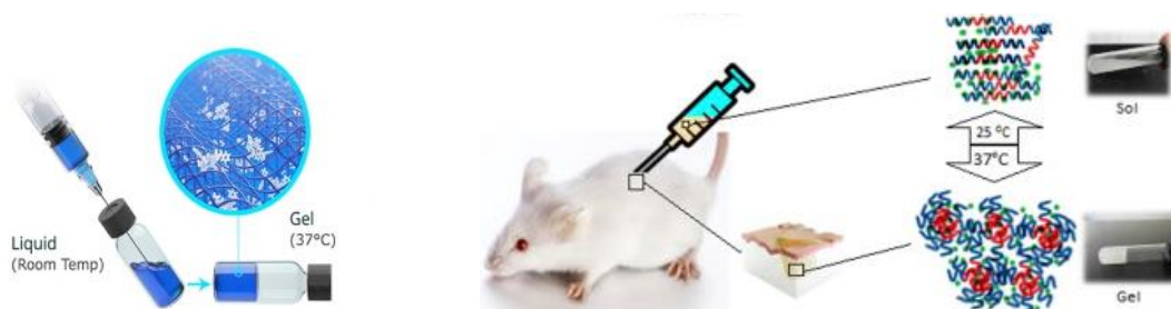
Figure 2.2: Illustration of thermoresponsive hydrogels which undergo gelation at body temperature. Adapted from Shaker et al [27].
