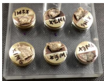
Figure 3.11: Representative photo of lyophilised hydrogels coated by a thin layer of Au prior to SEM analysis. Hydrogels were coated using an Edwards Au coater under Ar atmosphere.
