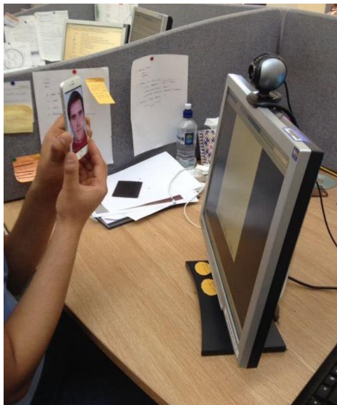
Figure 3.12: An impostor holding a displayed photo and attempting to follow the challenge during the simulated spoofing attack
