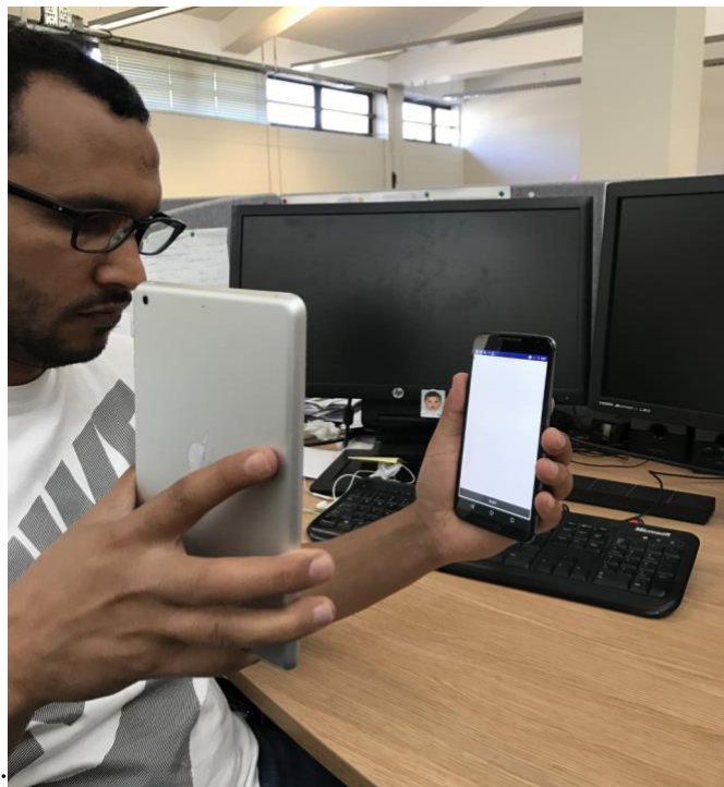
Figure 5.6: An impostor holding a displayed photo and attempting to follow the challenge during the simulated spoofing attack
