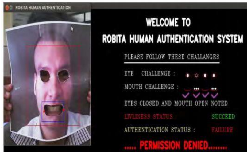
Figure 2.42: Spoof attack detected by the system in [131]
