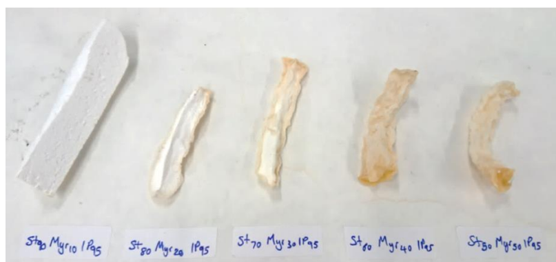
Figure 6.17 - Showing the 5 myrcene containing pHIPes (left to right: St 90 Myr 10 5XL, St 80 Myr 20 5XL, St 70 Myr 30 5XL, St 60 Myr 40 5XL, and St 50 Myr 50 5XL) immediately after being removed from the vacuum oven after drying at 45 °C.
