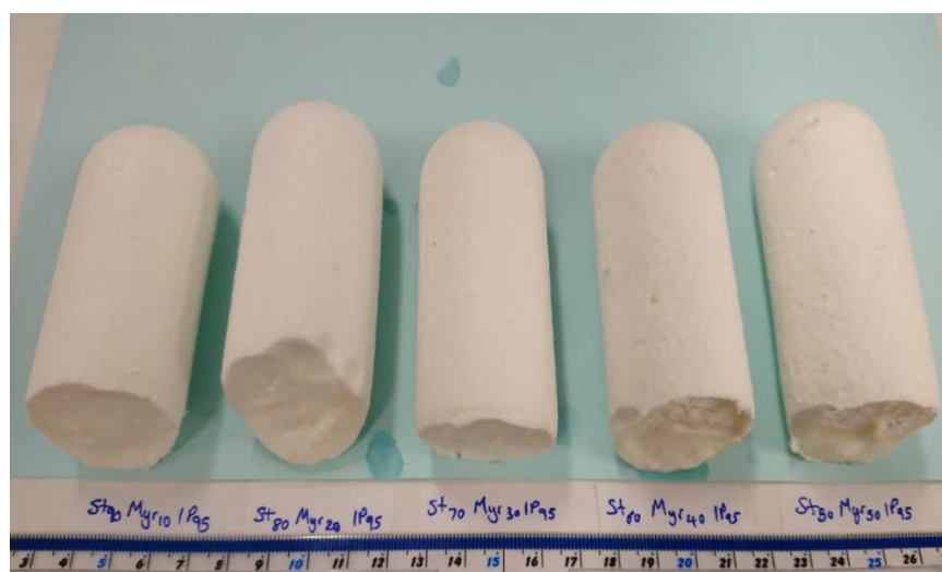
Figure 6.13 – A picture of the 5 myrcene containing pHIPes ( St_{90}Myr_{10}1XL , St_{80}Myr_{20}1XL , St_{70}Myr_{30}1XL , St_{60}Myr_{40}1XL , and St_{50}Myr_{50}1XL ) immediately after being removed from the curing tubes.
