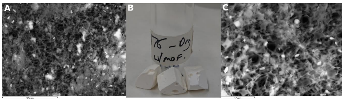
Figure 5.10 – SEM images of the DUT-HIPE (A and C) with an image of the formed composite in the middle (B).
