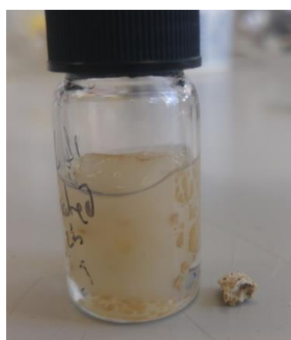
Figure 4.22 - On the left is a 7 ml vial showing swollen sulfonated-HIPE in water and to the right is an equivalent dry mass of the polymer on the right.
