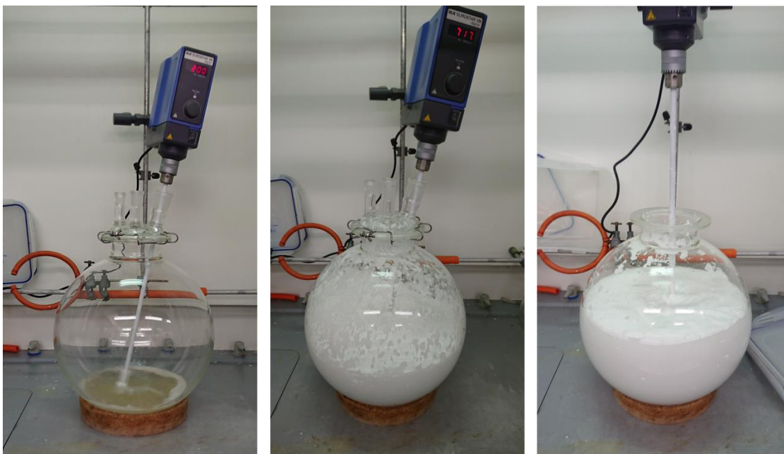
Figure 4.2 – Left; the set up for the mixing of the large scale pHIPes (20 L reactor), centre; mixing for the emulsion after addition of the first 25 % internal phase, right; the emulsion after addition of all internal phase.
