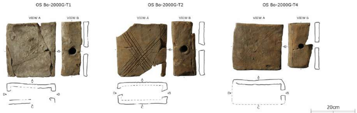
Fig 71: Three of the tubuli recovered from the post-Roman level in connection to the robber trenches of the bath house and most likely originating from this building. They demonstrate different sizes and scoring or combing patterns to give the superimposed plaster a better grip.
