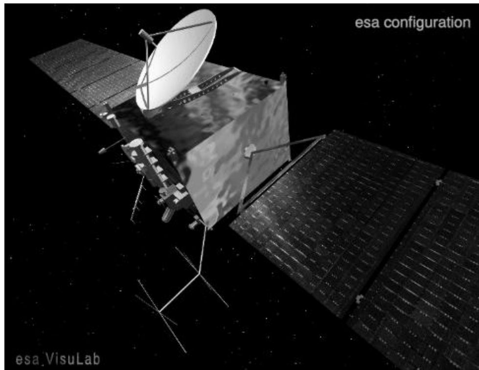
Figure 1.3. ESA Visulab computerised image of the Rosetta Orbiter (from Visulab web site at www.estec.esa.nl/visulab.html , 1996). The spacecraft bus is derived from a communications satellite.
