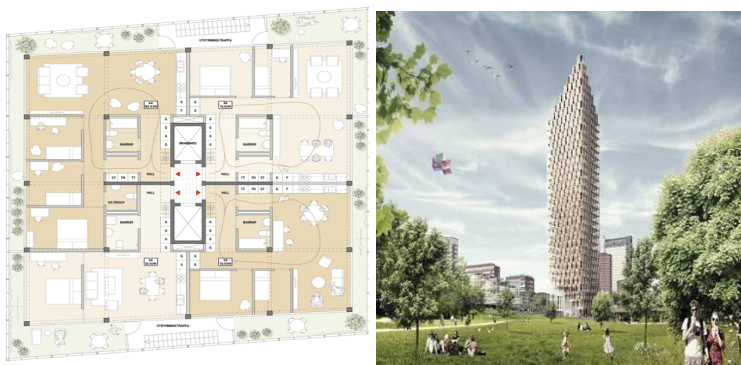
Figure 3.6: Typical floor plan and three-dimensional view of proposed 34-storey timber housing in Stockholm indicating articulated facade with provision for roof garden on each floor, that is, the individual balconies to each flat (C.F. Moller Architects, 2014).
