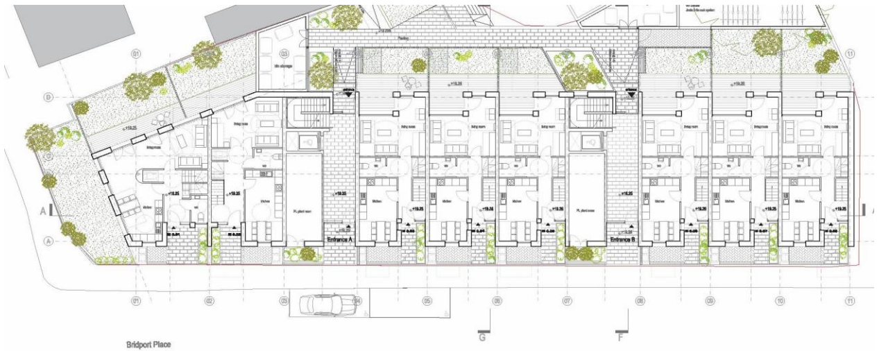
Figure 5.3: Ground floor plan of Bridport House showing the linear arrangement of the internal spaces of the maisonettes with front entrance doors, exit doors and private outdoor spaces at the rear side of the development including the bicycle sheds for the residents.
