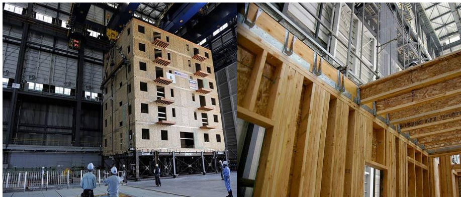
Figure 3.3: Testing of a prototype earthquake resistant prefabricated timber multi-storey house developed at the Hyogo Earthquake Engineering Research Centre in Japan to reduce the effect of earth movement and frequent seismic actions on houses (Inhabitat, 2014).
