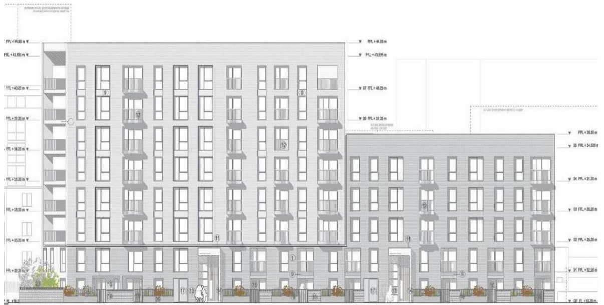
Figure 5.6: Street elevation (east facing) of Bridport House in Hackney showing eight-storey and five-story block of apartments with floor to ceiling height windows for ventilation and natural lighting and arrangement of balconies for relaxation and other purposes.
