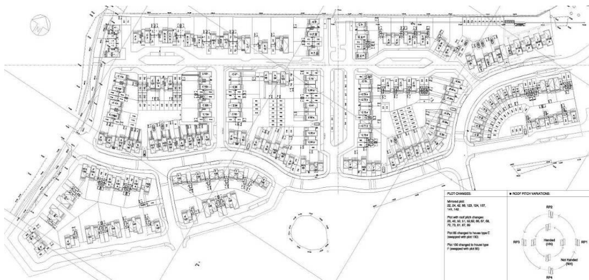
Figure 5.12: Site plan of Oxley Woods showing overall layout of the prototypes positioned at different orientations with private outdoor spaces at the back of the houses and good road networks to access the development (Richard Stirk Harbour & Partners- RSHP).
