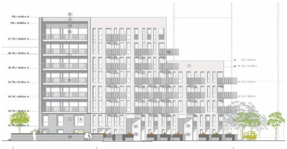
Figure 5.7: South facing elevation of Bridport House in Hackney showing the eight-storey and the five-story block of apartments.
