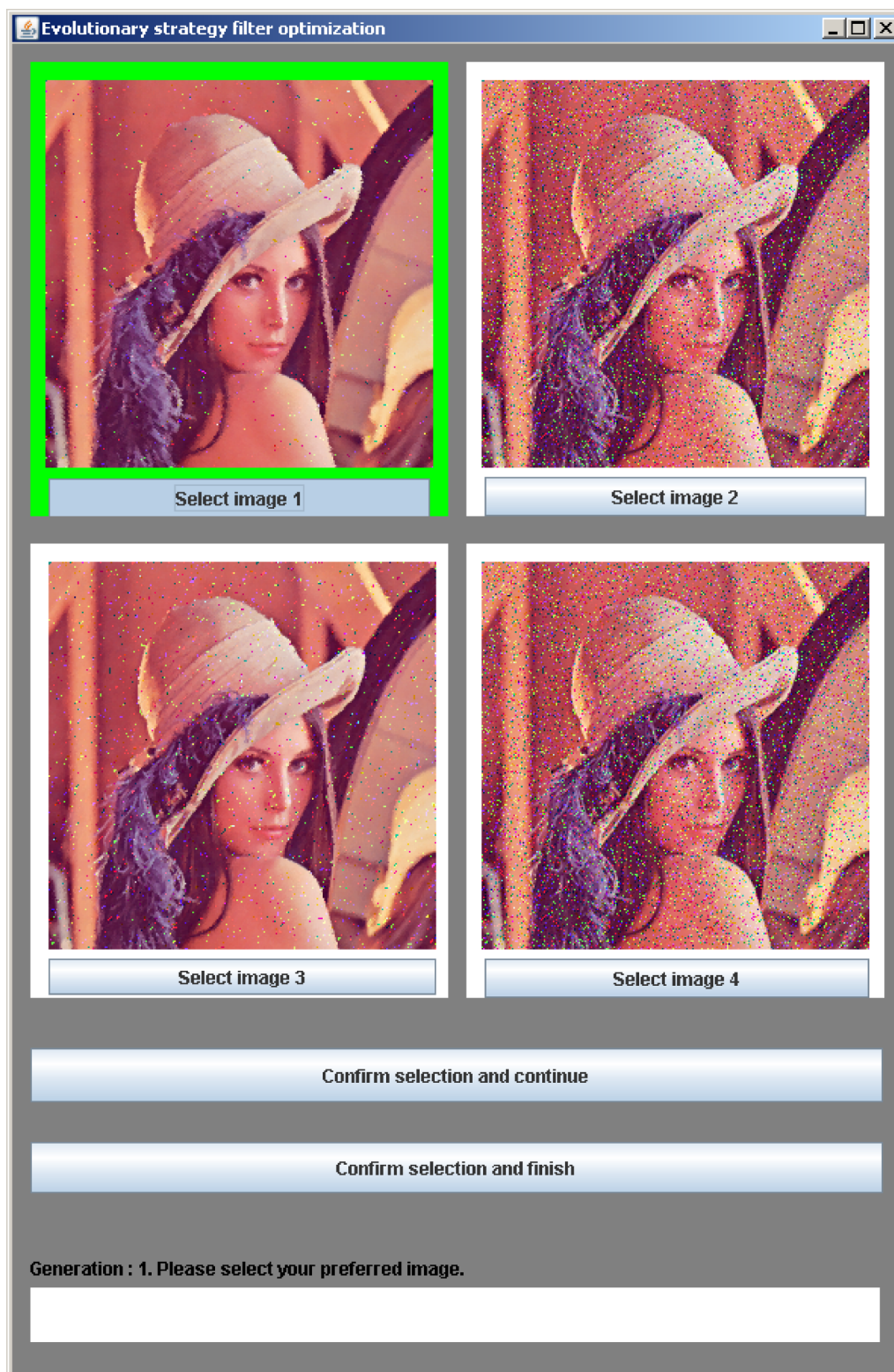
Figure 3.2: Screenshot of the user interface for the development of the filters in the noise removal experiment
