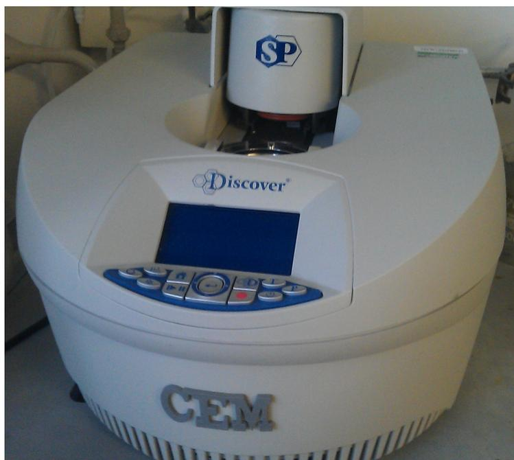
Figure 5: Image of the microwave oven synthesiser used for the experiments within this thesis.
