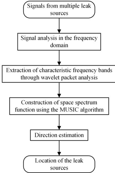
Fig. 1. Key steps in the localization method.
