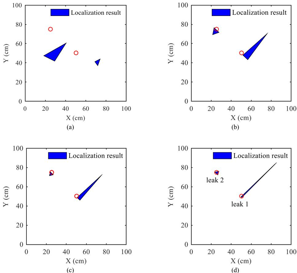
Fig. 15. Localization results corresponding to different leaking pressure. (a) 0.05 bar. (b) 0.1 bar. (c) 0.15 bar. (d) 0.2 bar.
