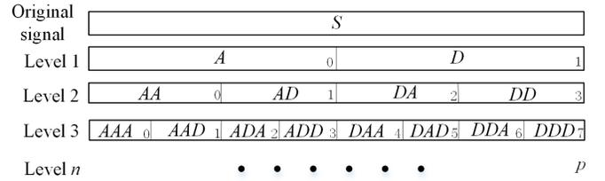
Fig. 2. N-level wavelet packet decomposition.
