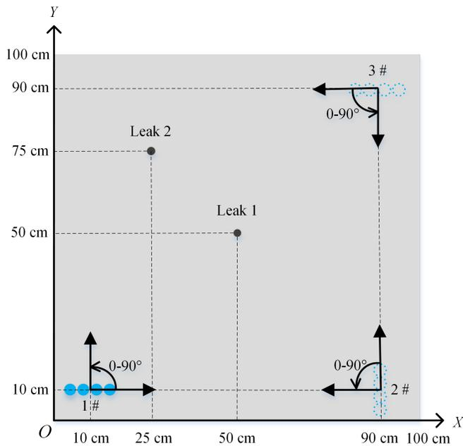
Fig. 6. Arrangement of the sensor array.
