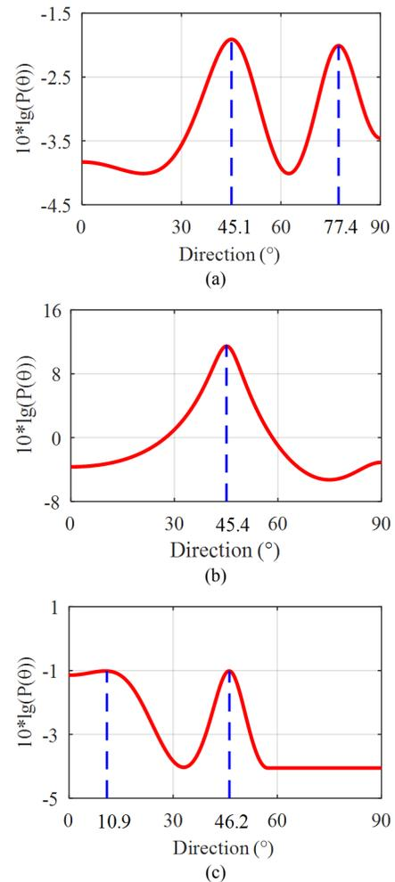
Fig. 11. Directional identification of the array at different locations 1#. (a) Location. (b) Location 2#. (c) Location 3#.
