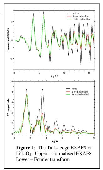
was  $700 \times 700$  microns. Powdered samples were mixed with cellulose as a diluent and pressed into 13 mm diameter pellets. The spectra were normalized in Athena and fitted to scattering models in R-space produced by FEFF in Artemis [24].
