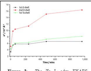
**Figure 2**: The Ta L<sub>3</sub>-edge EXAFS Debye-Waller factors for LiTaO<sub>3</sub> as a function of milling time.
