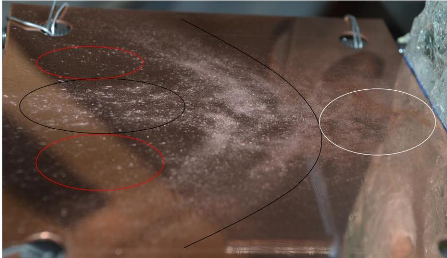
**Figure 37 - Image of the secondary ejecta pattern. The fan arm can be seen bounded by the curved black line, the black circle shows the high up central area of cratering, the two red circles show the pitting between those two regions, and the white circle shows the area that had some kind of trails present below the fan centre.**
