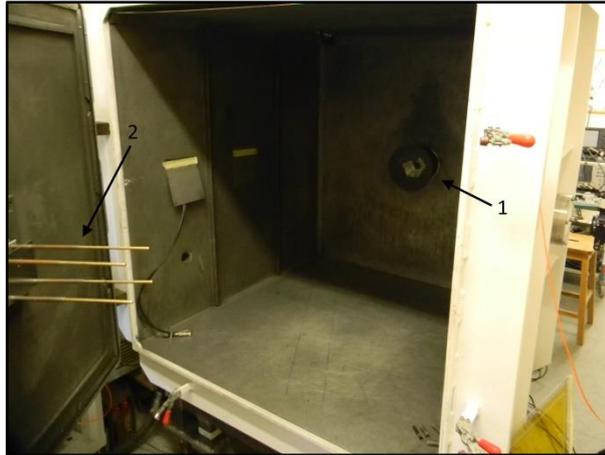
Figure 2 - Image showing the inside of the Target Chamber: (1) The connecting tube between the Blast Tank and the Target Chamber through which the projectile travels, (2) Target Mounting Bracket attached to the Target Chamber door where the user-defined target can be fitted.
