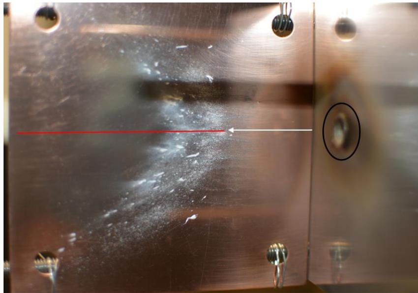
**Figure 11 - Image showing the impact crater (within the black circle) and the copper witness plate with the distinct sideways 'V' shaped secondary ejecta pattern. The red line has been placed to indicate the approximate visual centre of the 'V' pattern, and the white arrow indicates where the projectile matter began within the 'V' pattern (using a Scanning Electron Microscope) from the base of the witness plate.**
