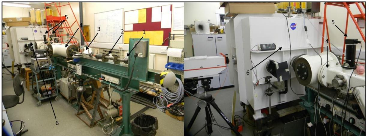
**Figure 1 - Labelled images of the Light Gas Gun showing its major components: (1) Powder Chamber, (2) Pump Tube, (3) Launch Tube, (4) Blast Tank, (5) Dual Laser Blanket connected to oscilloscope, (6) Target Chamber.**
