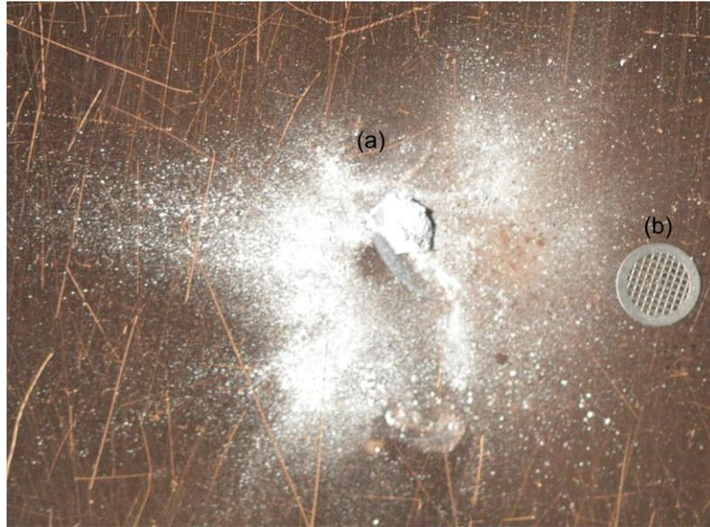
**Figure 28 - Image showing the burst-through ejecta with a small chunk of aluminium sticking out of copper witness plate at marker (a), and the 2.5mm size marker, (b).**
