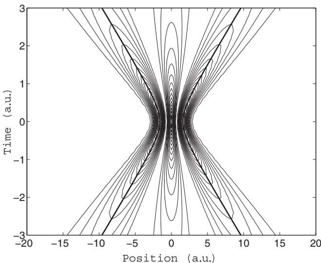
FIG. 1. Contour map of the density associated with the wave function of Eq. (2) as a function of time and space. This was evaluated for  $t_c = 1$  a.u. with  $n = 2$ . Superimposed on this are the hyperbolas given by Eq. (6).
