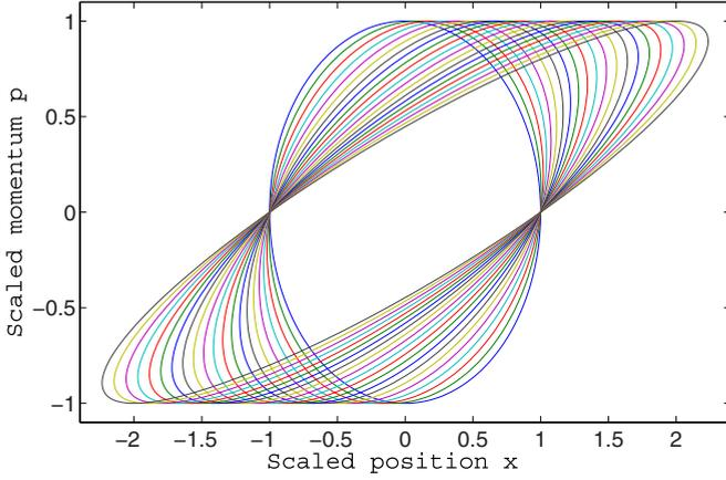
FIG. 2. (Color online) Phase-space curves ( $p$  vs  $x$  for the family of paths described by Eqs. (9) and (10). At  $t = 0$  this is a circle in phase space which shears into an ellipse as time proceeds.
