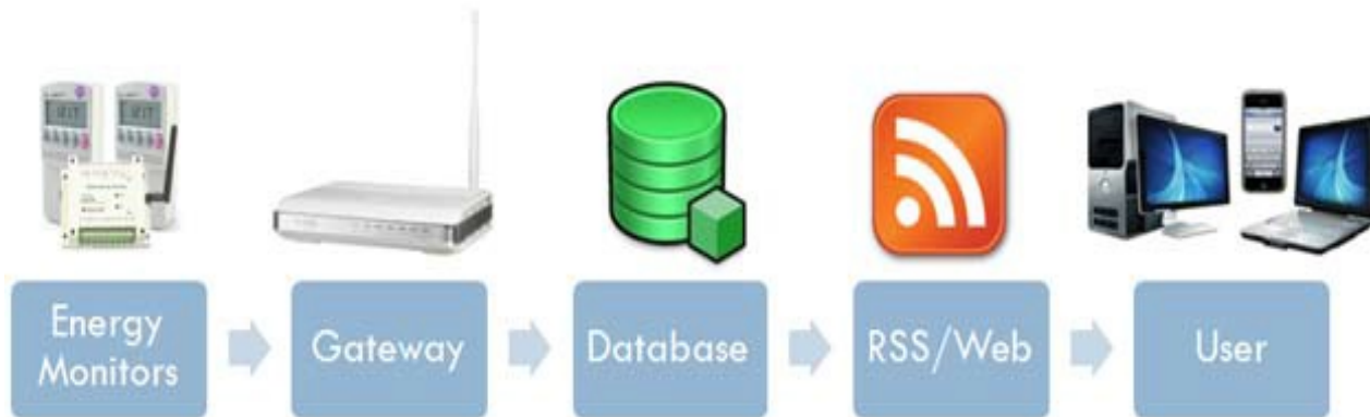
Figure 8. The flow of information from the electricity meters to a user display [19].
