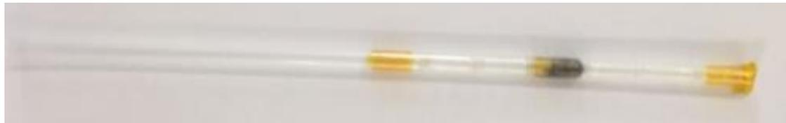
Figure 2.12 Picture of a sample ready for magnetometry measurements
