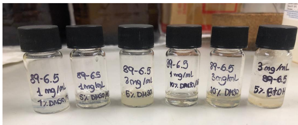
Fig. S99. Solubility studies of poly1 at different concentrations (1 mg/mL and 3 mg/mL) and different percentages of DMSO in water (1 %, 5 % and 10 %) and in 5 % MeOH in water at a concentration of 3 mg/mL.
