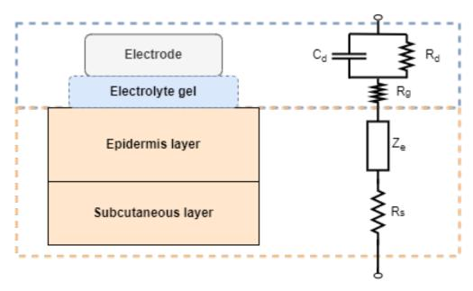
FIGURE 2.5: Equivalent circuit for a metal electrode.
