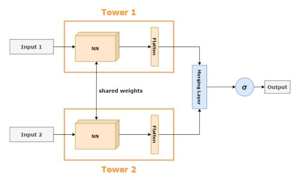
FIGURE 5.9: Generic Siamese network. In the merging layer, a distance metric function is executed to calculate distances between pairs.
