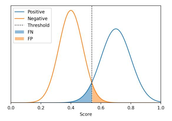
FIGURE 2.1: An example of scores distribution from genuine and forgery samples. Blue and orange filled areas represent the classification errors of the system, given the optimal threshold.
