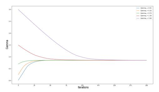
Figure 4.4: Weight update over training from different initial values. For higher values, more iterations are needed to reach convergence to the optimal value.
