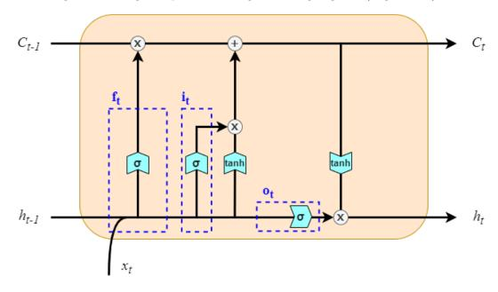
FIGURE 3.5: LSTM cell diagram, describing the various gates and input-output connections.
