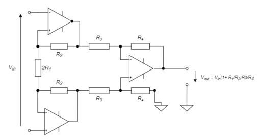
FIGURE 2.6: Schematics of a generic instrumentation amplifier. The first two buffers are connected to the electrodes.
