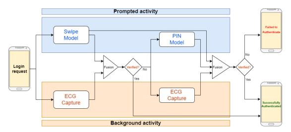
FIGURE 2.8: All the stages of the framework. Pin and the second ECG recording are prompted only after a failure from the previous modalities.
