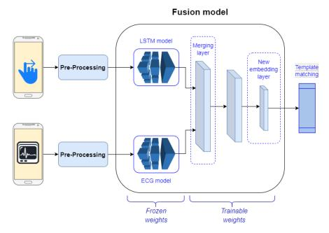
FIGURE 6.5: Two modalities fusion at model Level. Original models with frozen weights are combined with a merging layer. The remaining layers of the new architecture are the only one with trainable weights. The training is conducted with batches of paired data from the same class.
