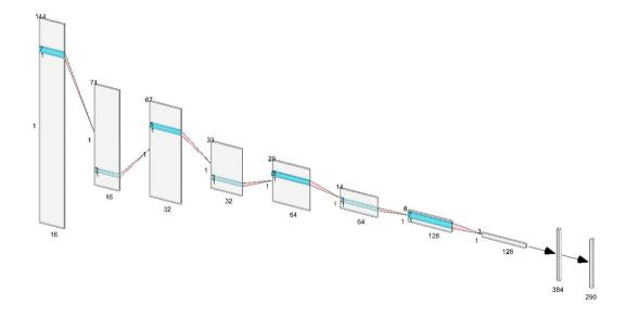
Figure 5.8: Visualization of the DeepECG-like deep learning model. Blue sections inside layers represents the filters. Numbers describe layers and filters dimensions (height, width and depth).
