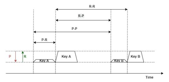
FIGURE 4.1: Keystroke time intervals based on Press (P) and Release (R) events.
