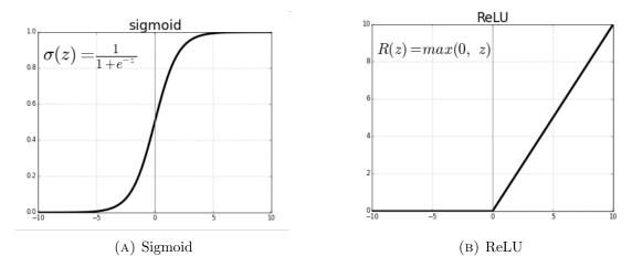
Figure 3.4: Activation functions. Sigmoid (A) and ReLU (B)
