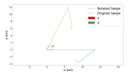
FIGURE 3.3: Example of Swipe projected on the x-axis before using the shifted zero crossing. x and v are the two versors. Without the transformation, the original swipe wouldn't be rejected.
