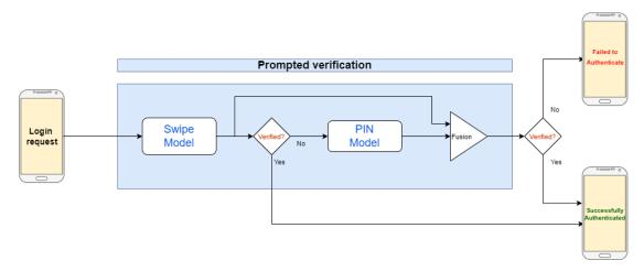
FIGURE 4.3: Adapted framework of the verification pipeline for Swipe and PIN. PIN verification is prompted only after a swipe failure, which means that the fusion cannot happen before that event.
