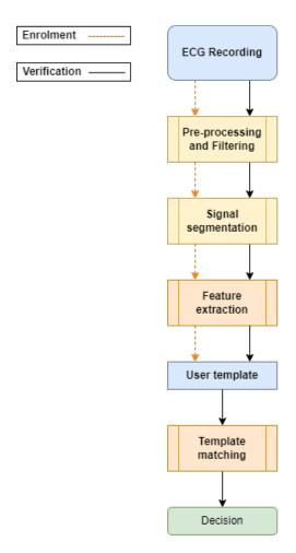
Figure 5.3: Generic framework for ECG verification, regardless of the model used for decision making. This block diagram is valid for each subject on a non-continuous authentication.
