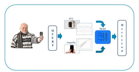
FIGURE 2.7: Multi-modal authentication, combining the three modalities (Swipe,Pin and ECG) in this study. The user tries to login to a service provider (e.g. a bank account) and the server requests a multi-modal biometric authentication.
