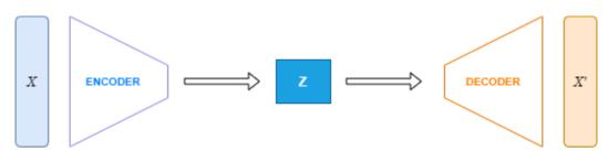
Figure 5.10: Generic structure of an autoencoder. X is the output, Z the latent space and X' the reconstructed output.
