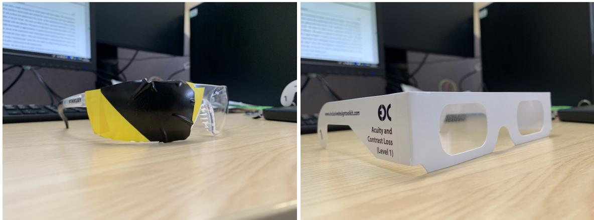
(a) Glasses to simulate semi-neglect condition. (b) Glasses to simulate short-sightedness condition.
