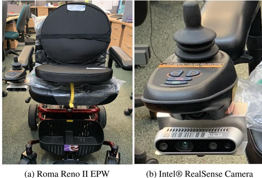
Fig. 3.1 The camera is installed beneath the EPW’s joystick so that no interference with the users’ legs can obstruct vision.
