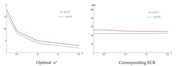
Fig. 4. Optimal n<sup>\*</sup> and corresponding Expected Cost Rate when Mode I is repairable when Mode I is repairable.
