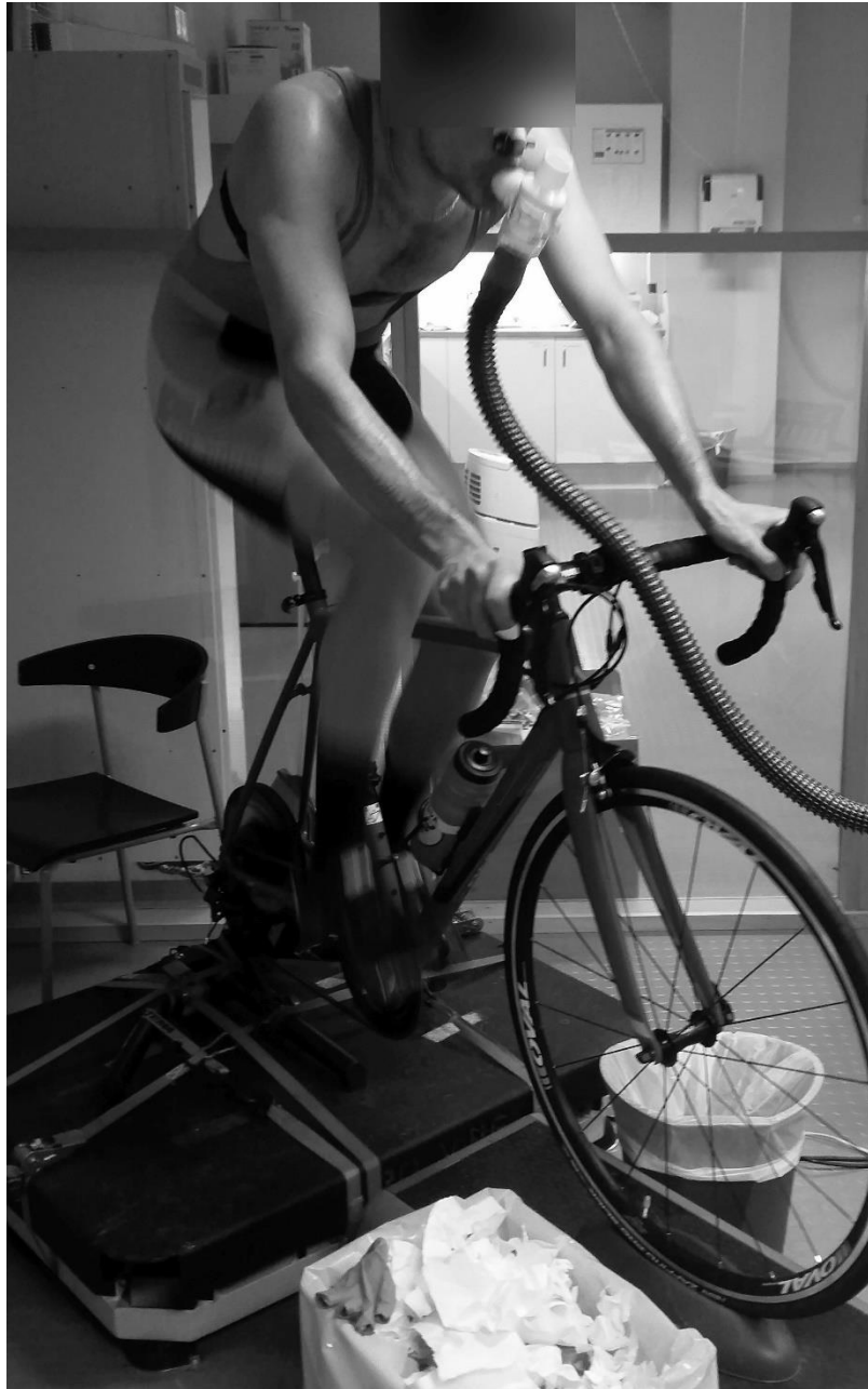
Figure 1 Ergometer set-up. The bike frame is mounted on the cycle ergometer, which is attached to the vibration platform with ratchet straps. The vibration platform is screwed on the floor. The front wheel of the bike is on a riser block, which is on top of a fitness step. The cyclist is breathing through a mouthpiece connected to the metabolic cart.
