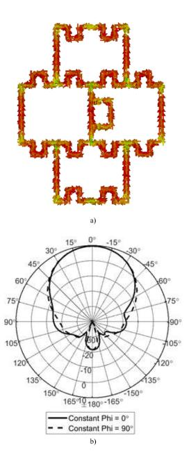
Fig. 5. Simulated pattern of current (a). Simulated radiation gain for the meandered 4-cell wearable GAA (b).
