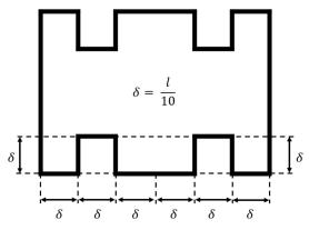
Fig. 4. Meandered GAA Cell
