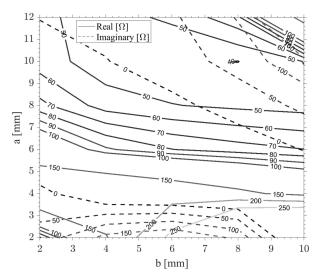
Fig. 3. GAA matching chart by varying T-match shape factor a, b.
