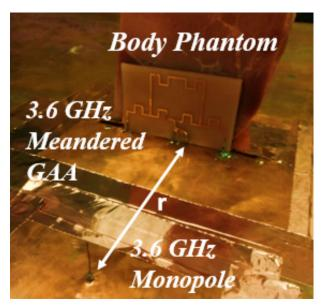
Fig. 6. Experimental setup for measuring the input impedance and gain of half-grid when attached onto a roasted pork phantom; probe monopole length  $l=20\,$  mm and  $r=13\,$  cm.
