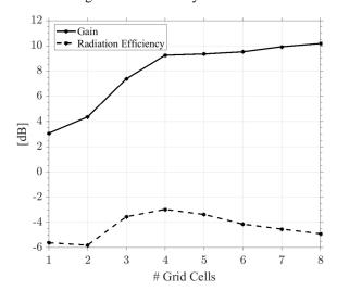
Fig. 2. Simulated upper-bound gains and efficiency of wearable grids vs. number of grid array cells. Maximum efficiency is achieved by a 4-cell grid with 7 radiating elements.
