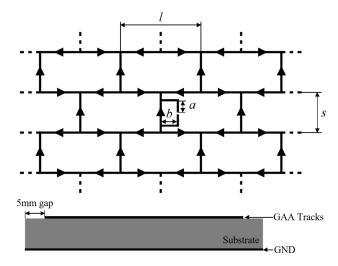
Fig. 1. Multi-cell GAA structure featuring T-match feeding network with indication of the typical current pattern and cross-sectional view.
