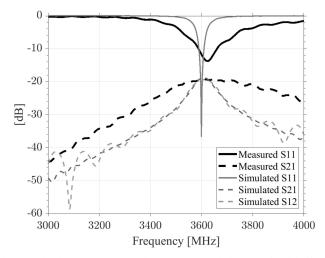
Fig. 7. Simulated and Measured S-parameters of the meandered half-grid sourced by a test monopole.
