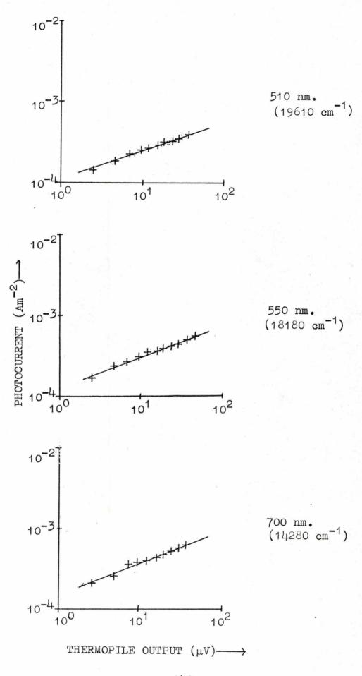
FIG: (5.36) PHOTOCURRENT INTENSITY DEPENDENCE PLOTS FOR ZINC PHTHALOCYANINE IN DRY AIR
