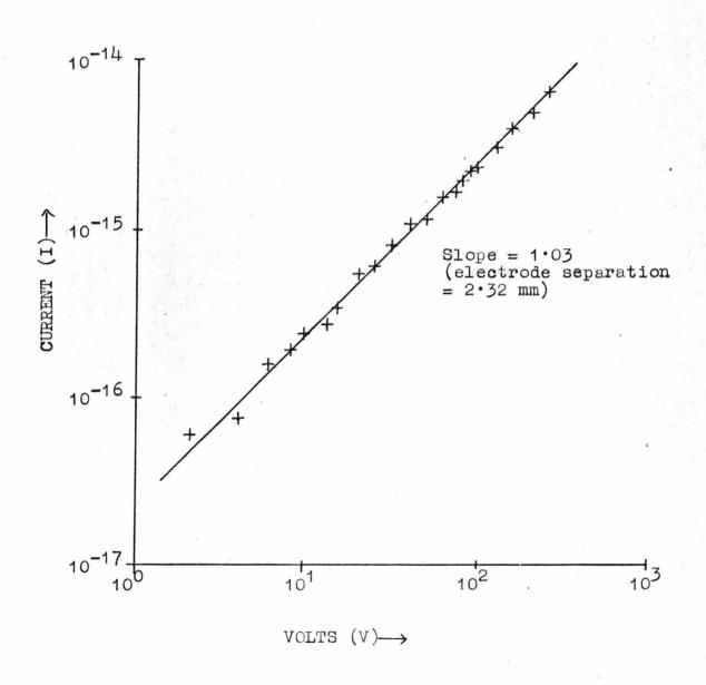
FIG: (6.27) ACTIVATION ENERGY PLOT FOR COPPER OXINATE IN A HIGH VACUUM
