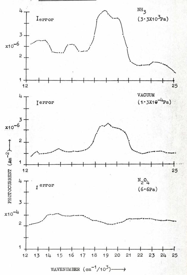
FIG: (5.25) PHOTOCONDUCTION SPECTRA OF ZINC PHTHALOCYANINE
