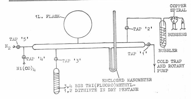
Purification of the dark red malodorous liquid was carried out by repeated distillation (10 times), and resulted in a malodorous straw yellow liquid. It was found that after purification the 3,4bis(trifluoromethyl)-1,2-dithiete readily dimerised (in a few hours) and it was found that this dimer could not be reacted with nickel carbonyl to form bis[cis-3,4bis(trifluoromethyl)-1,2-dithiete]nickel, hence the 3,4bis(trifluoromethyl)-1,2-dithiete was only purified immediately before use.
