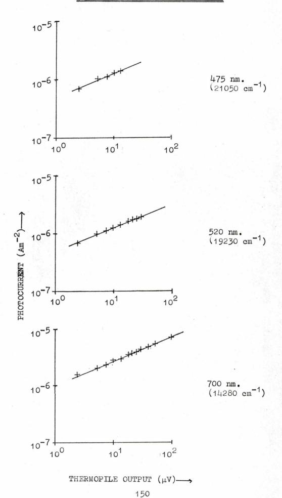
FIG: (5.37) LEAD PHTHALOCYANINE PHOTOCONDUCTION SPECTRA
