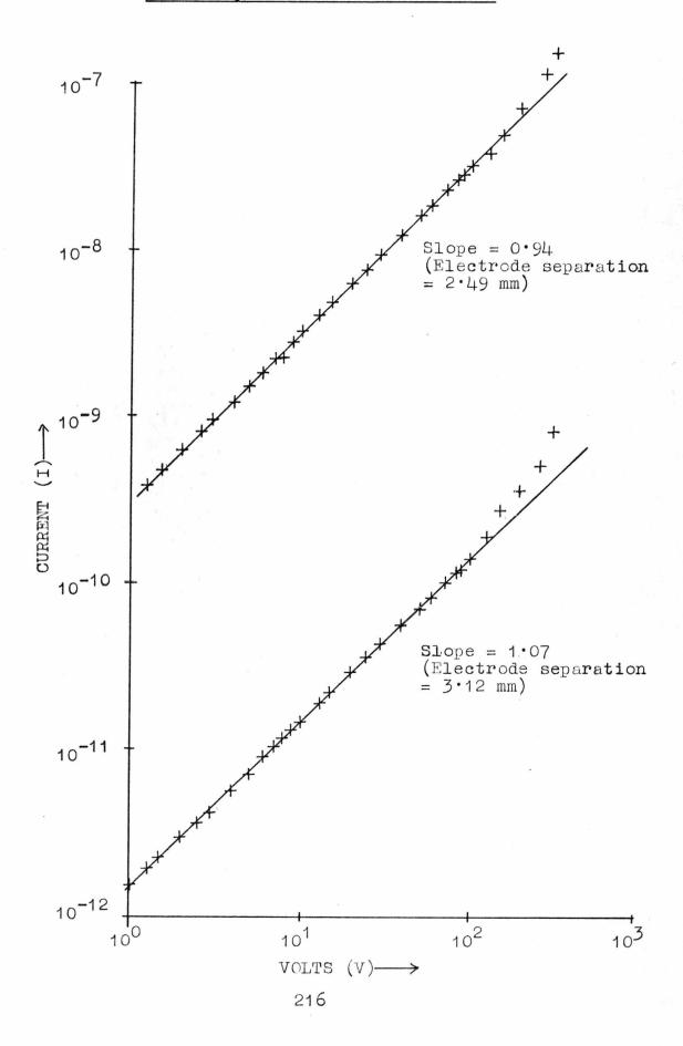
FIG: (6.24) ACTIVATION ENERGY PLOTS FOR BIS[CIS-3,4-BIS(TRIFLUOROMETHYL)-1,2-DITHIETE]NICKELOUND IN DRY NITROGEN
