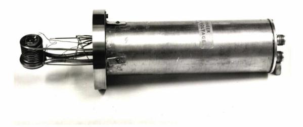
FIG: (4.14) DETAIL OF A MOUNTED CRYSTAL
