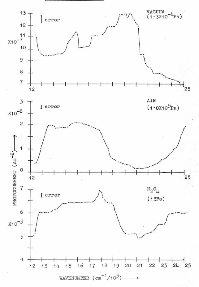
FIG: (5.26) PHOTOCONDUCTION SPECTRA OF COPPER PHTHALOCYANINE
