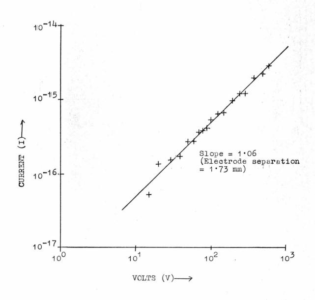
FIG: (6.26) OHMIC PLOT FOR PALLADIUM OXINATE IN A
