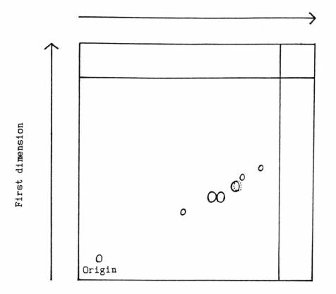
Fig. 4.15. The plate spotted with concentrated <u>Pen. claviforme</u> culture filtrate ( ) or patulin ( ...... ) and developed in toluene/ethyl acetate/formic acid (5:4:1, v/v) in the first dimension and chloroform/methanol (4:1, v/v) in the second. Components were located by spraying with 0.5% (w/v) 3-methyl-2-benzothiazolinone hydrochloride in distilled water followed by heating at 105°C for 10min. Chromatograms were traced 24h after chemical and heat treatment.
