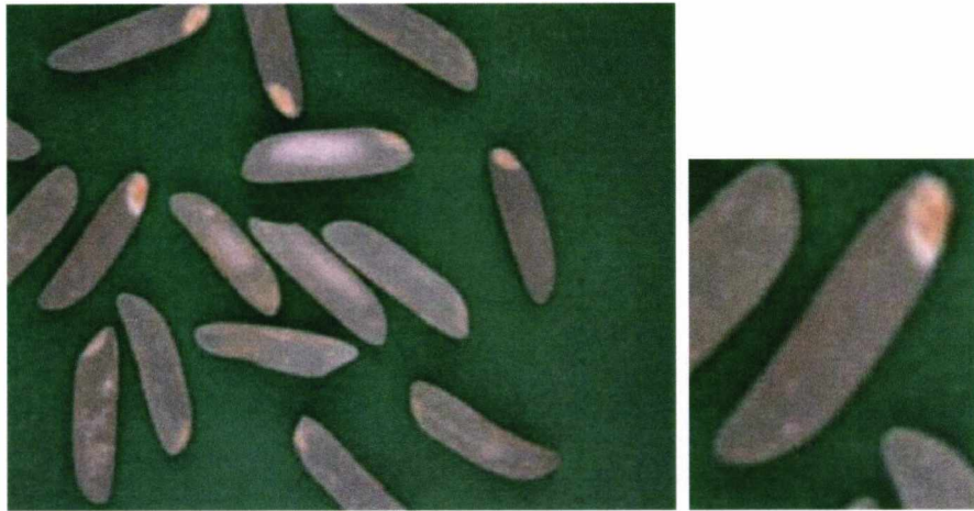
Figure 6.15. ROI and single object imaged with Celestron NexImage CCD.
