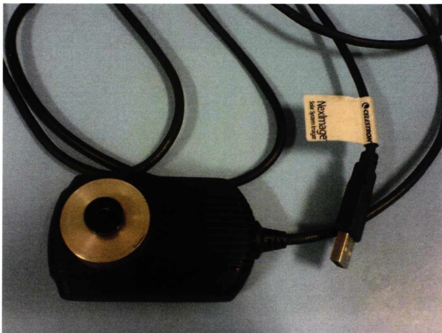
Figure 3.16. Celestron NexImage Dedicated CCD with custom lens mount.
