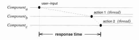
Component<sub>a</sub> controls the GUI that accepts user inputs.
