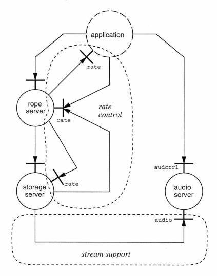
Figure 36: Structuring continuous media applications in terms of support for synchronisation and streams.
