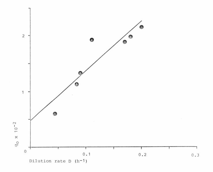
FIGURE 39: Determination of the Maintenance Coefficient for Ethanol Formation (Fermentation) from Glucose by 5D-cyc.
