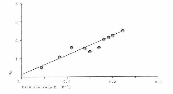
FIGURE 37: Determination of the Maintenance Coefficient for Carbon Dioxide Production (Fermentation) from Glucose by 5D-cyc.
