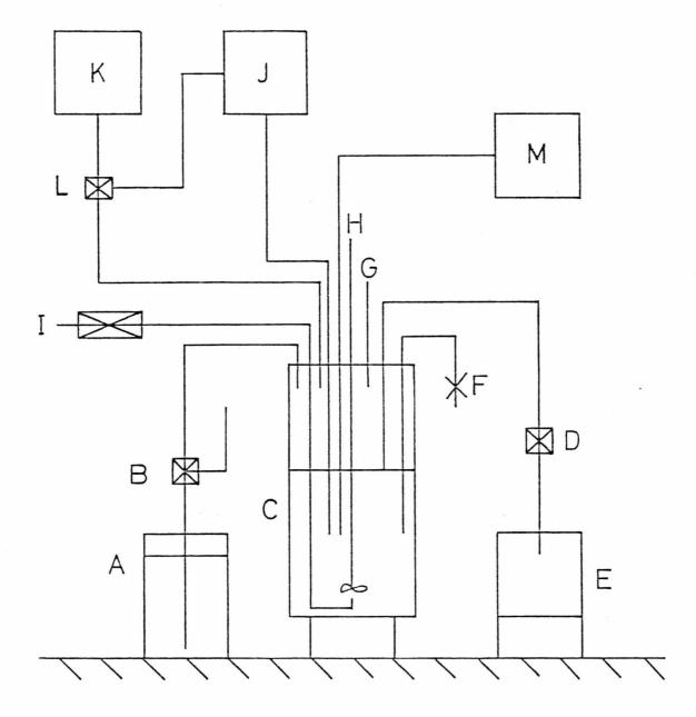
In the chemostat the growth rate of microorganisms is governed by the dilution rate (D) of the culture, where D = F/V; F = the flow rate (volume of fresh medium added to the culture vessel/unit time) and V is the volume of the culture. The dimension of D therefore is reciprocal time,  $h^{-1}$ . The change in the concentration of microorganisms is: change = growth - output (2) and since growth is  $\mu x$  and output is Dx (where x equals the concentration of organisms (g dry weight  $1^{-1}$ )
