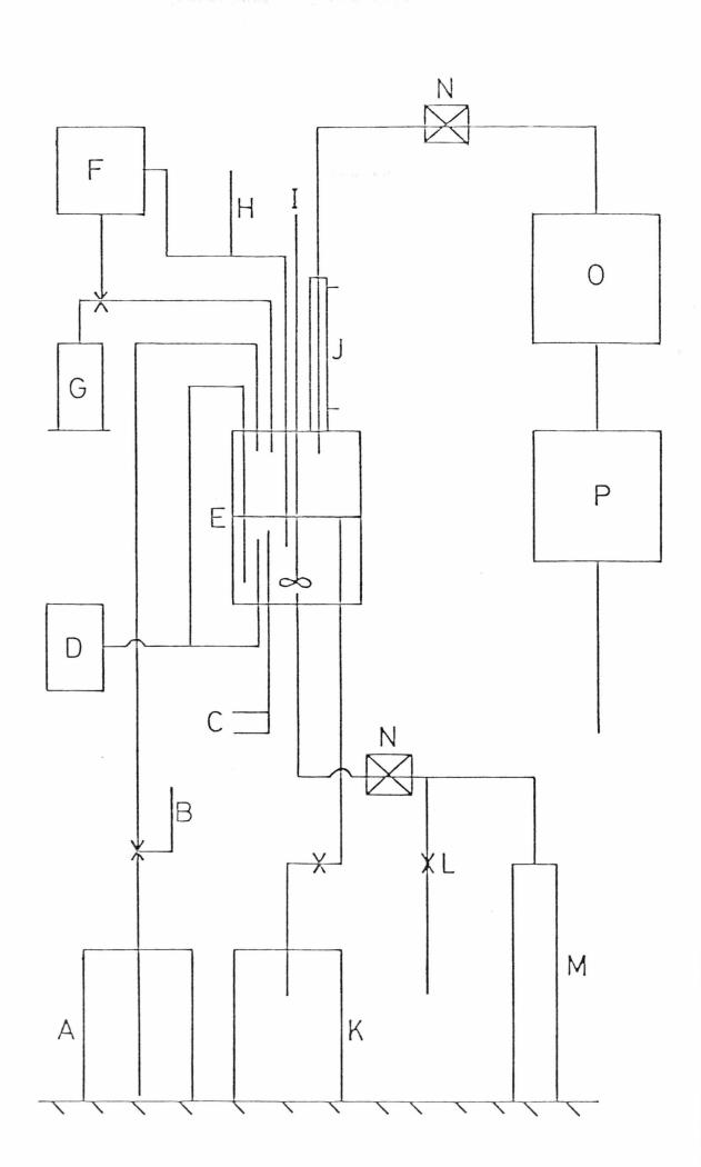
Temperature control was provided by a pulse ratio controller (Nobel Instruments Ltd.) using a 180 W, 240 V heating cartridge in conjunction with a cooling finger using circulating water at  $10^{\circ}$ C.
