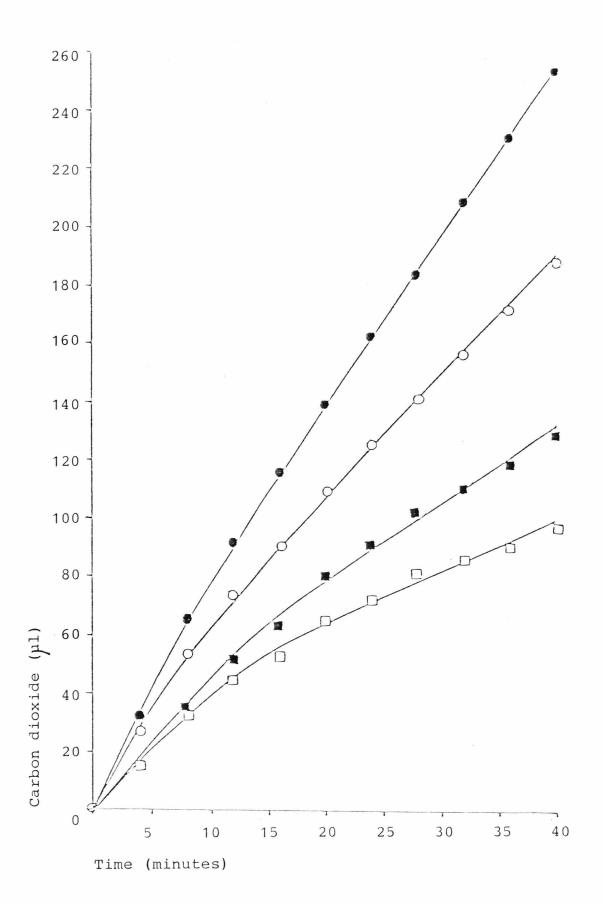
FIGURE 20: Effect of Ethanol on Fermentation in the Two Yeast Strains: Plot for Non-Competitive Inhibition Kinetics.
