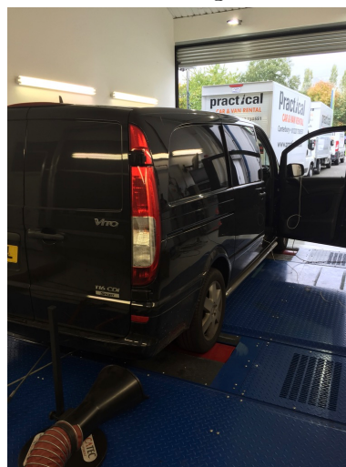
Figure .3.4.12 The Maha MSR500 Chassis Dynamometer in use.
