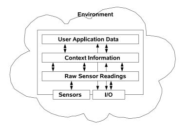
Figure 3.2: Abstract view of a sensor node architecture
