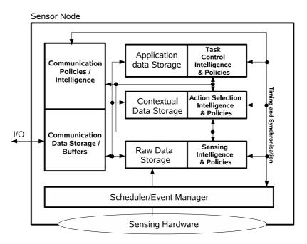
Figure 3.3: Functional/Architectural view of a sensor node
